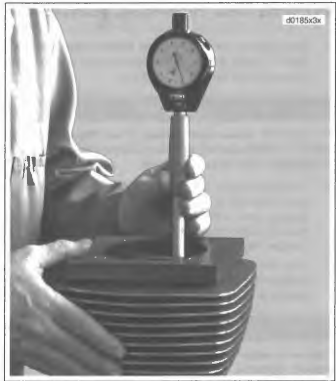
Figure 3-116. Measure For Out-of-Round and Taper
