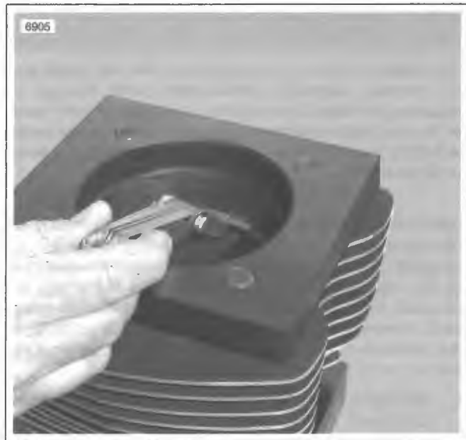
Figure 3-121. Measure Ring Gap
