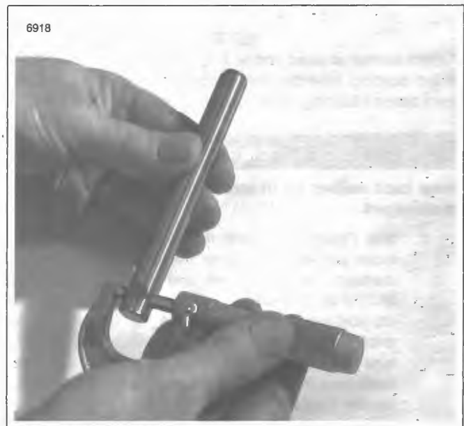
Figure 3-89. Checking Shaft to Support Plate Fit
