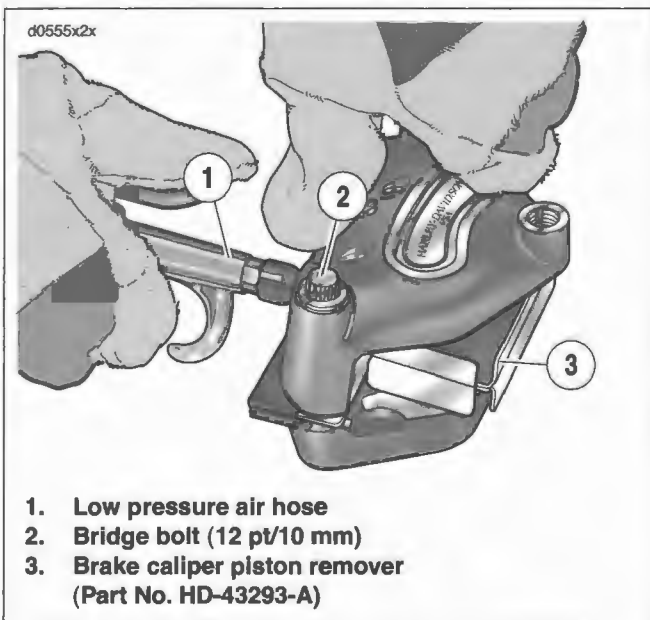
Figure 2-82. Removing Pistons
