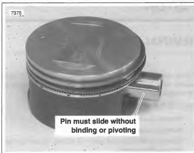
Figure 3-118. Piston Pin Clearance
