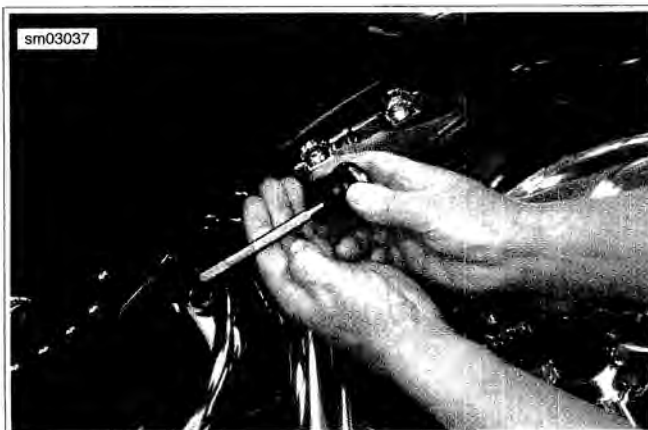
Figure 1-1. Checking Oil Tank Level
