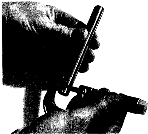
Figure 3-88. Checking Shaft to Support Plate Fit
