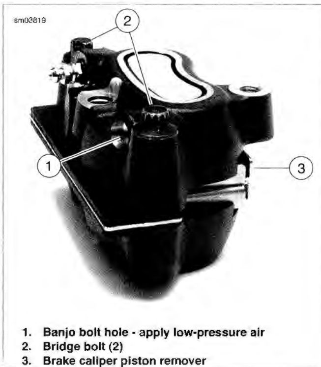
Figure 2-36. Removing Pistons
