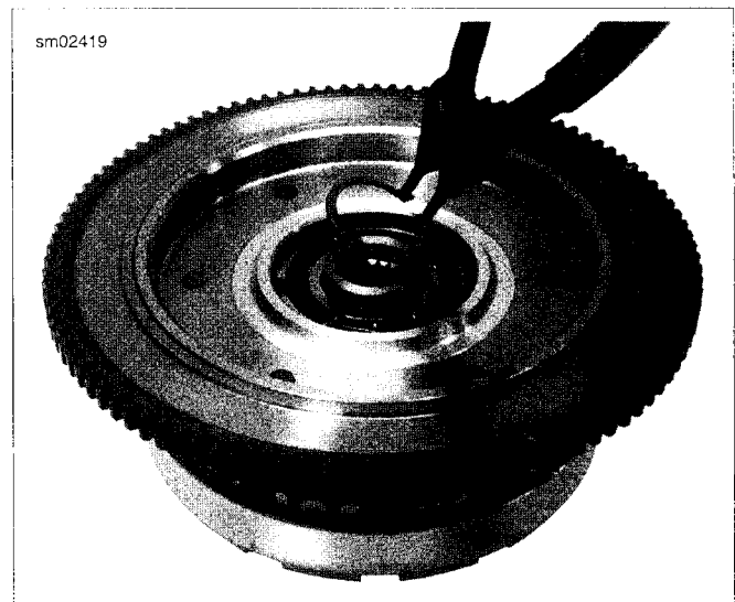
Figure 5-32. Clutch Hub Retaining Ring
