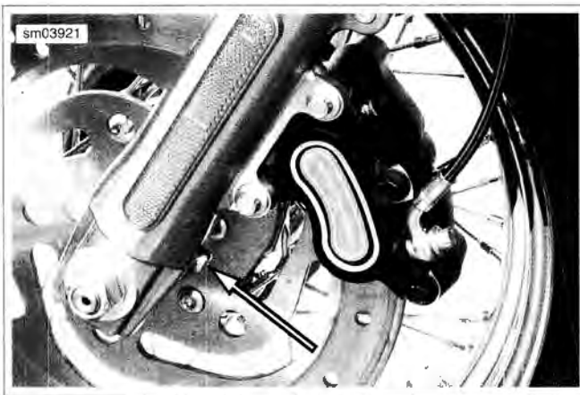
Figure 2-63. Fork Drain Screw: All Models Except FXCWC (Left Side Shown)
