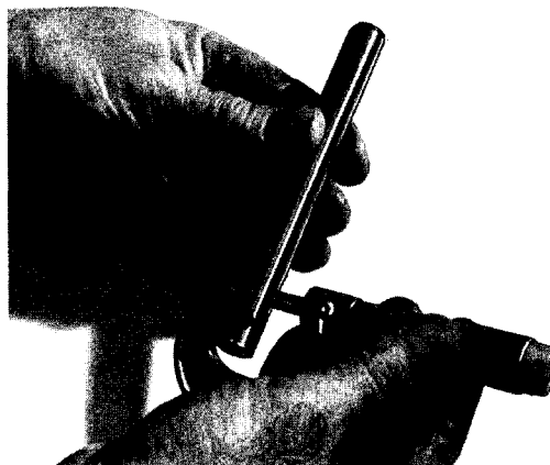
Figure 3-90. Checking Shaft to Bushing Fit
