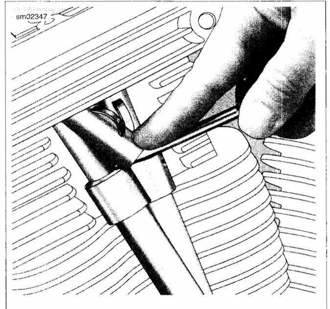
Figure 3-47. Install Spring Cap Retainers
