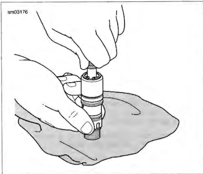
Figure 2-50. Compress Spring and Retaining Ring
