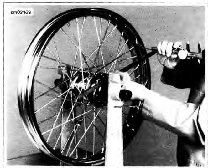
Figure 2-23. Front Wheel Hub Offset Dimension
