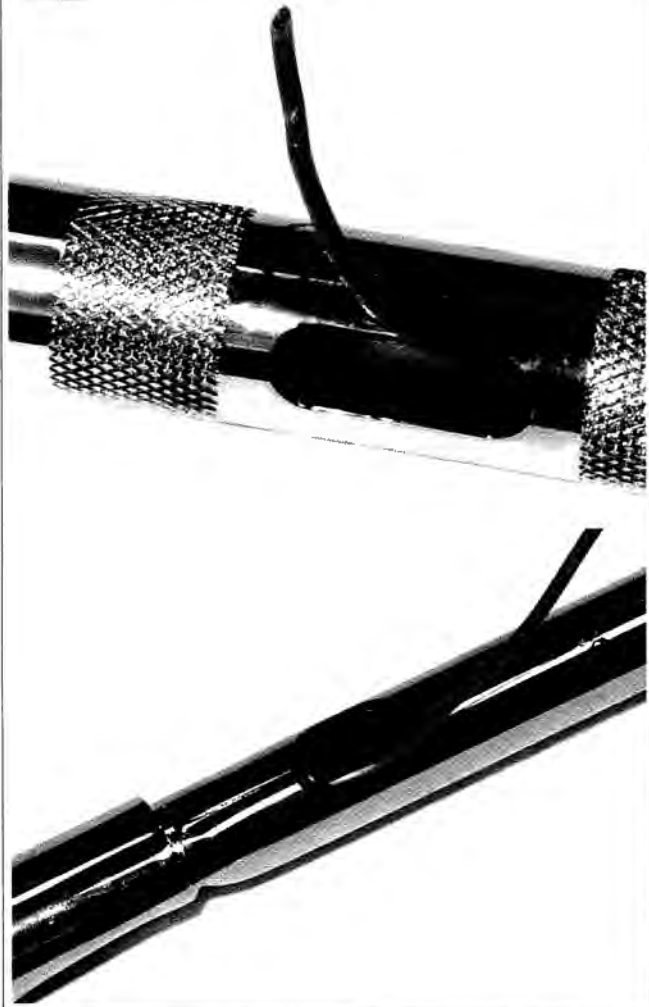
Figure 2-97. Wire Leader in Handlebars (handlebars removed from motorcycle)
