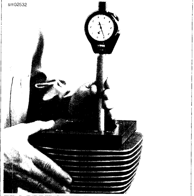
Figure 3-116. Measure for Out-of-Round and Taper
