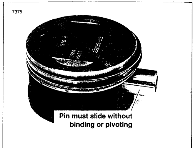
Figure 3-114. Piston Pin Clearance
