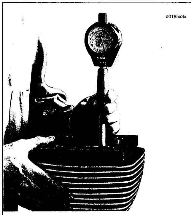
Figure 3-112. Measure For Out-of-Round and Taper
