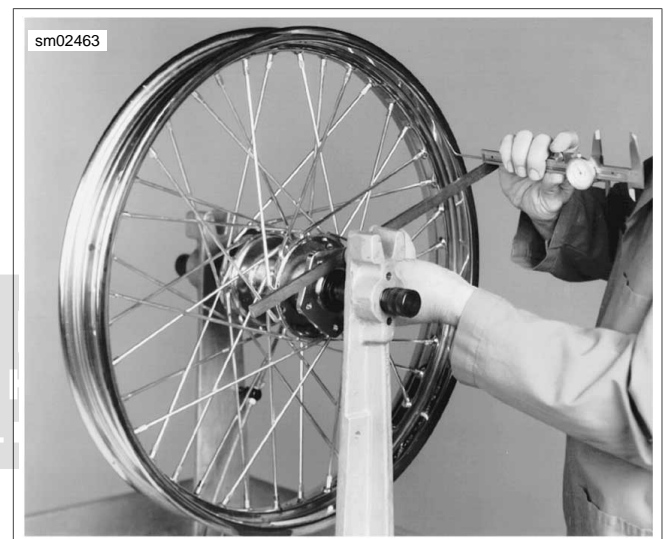
Figure 2-52. Front Wheel Hub Offset Dimension
