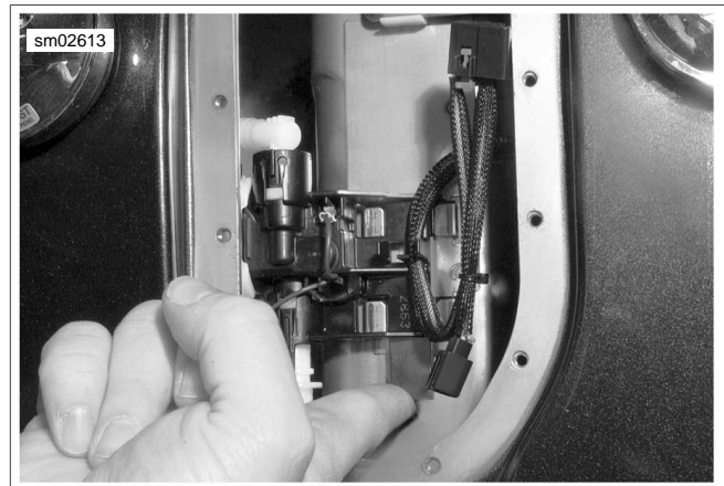
Figure 4-39. Fuel Pump Removal
