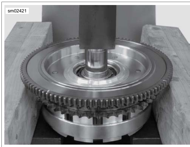
Figure 5-33. Pressing Clutch Hub From Bearing
