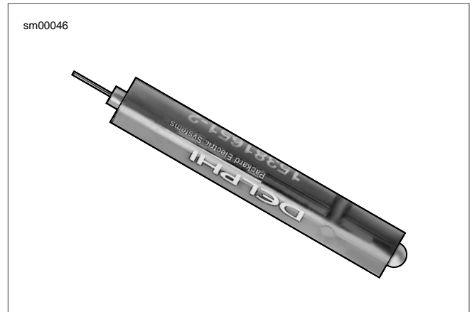
Figure A-47. Packard Micro 64 Terminal Remover (HD-45928)
