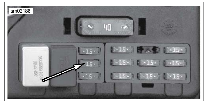
Figure 4-3. Fuel Pump Fuse
