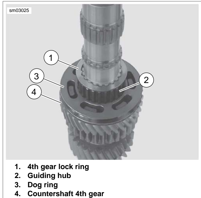
Figure 6-23. Countershaft Assembly
