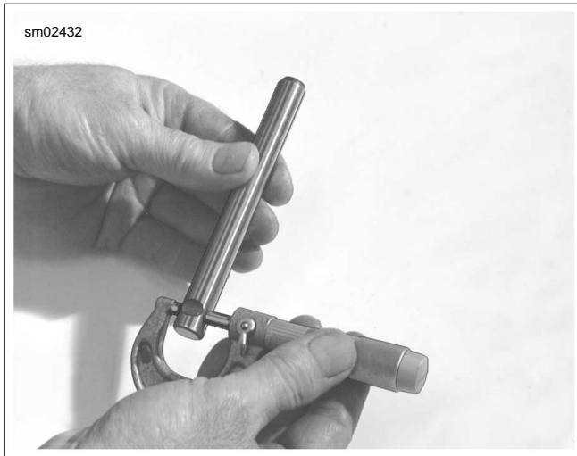
Figure 3-71. Checking Shaft to Support Plate Fit
