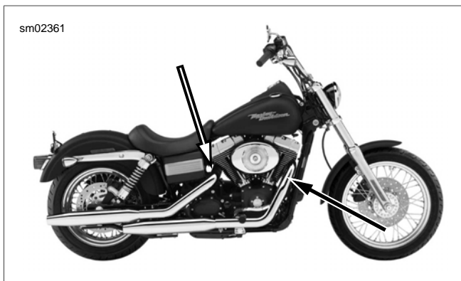
Figure 4-27. Oxygen Sensors (Inboard Side of Exhaust Pipes)
