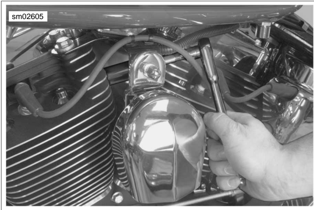
Figure 4-16. Engine Temperature Sensor Removal
