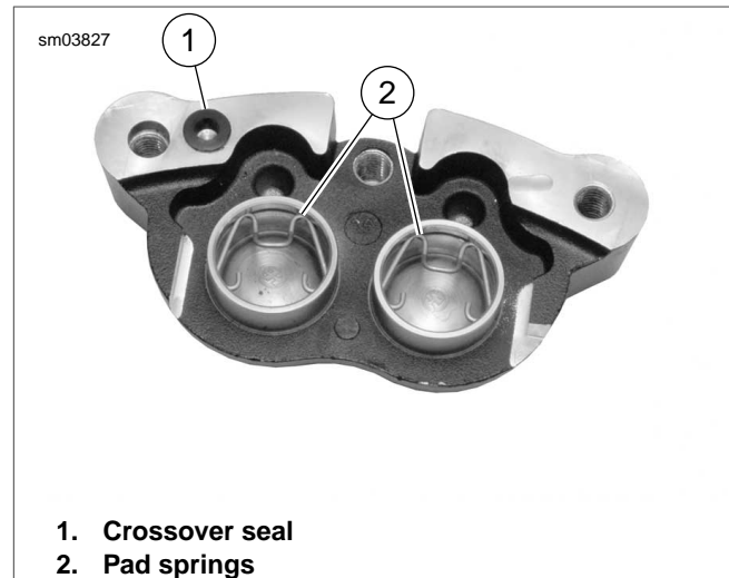
Figure 2-71. Front Caliper Pad Springs
