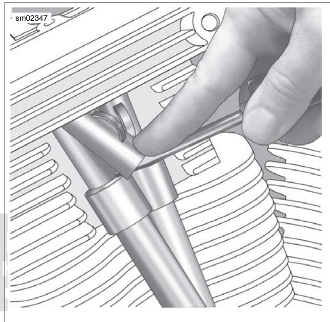
Figure 3-43. Install Spring Cap Retainers
