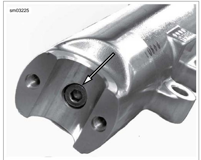
Figure 2-84. Seat Pipe Screw (right fork assembly)
