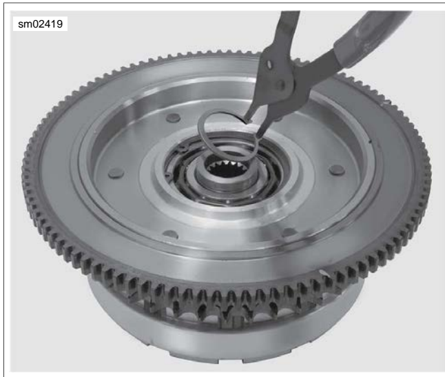
Figure 5-32. Clutch Hub Retaining Ring
