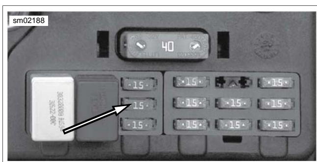
Figure 4-56. Fuel Pump Fuse
