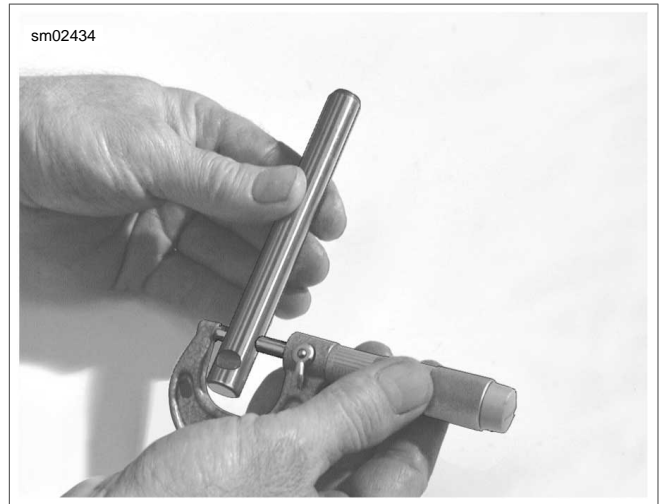
Figure 3-73. Checking Shaft to Bushing Fit
