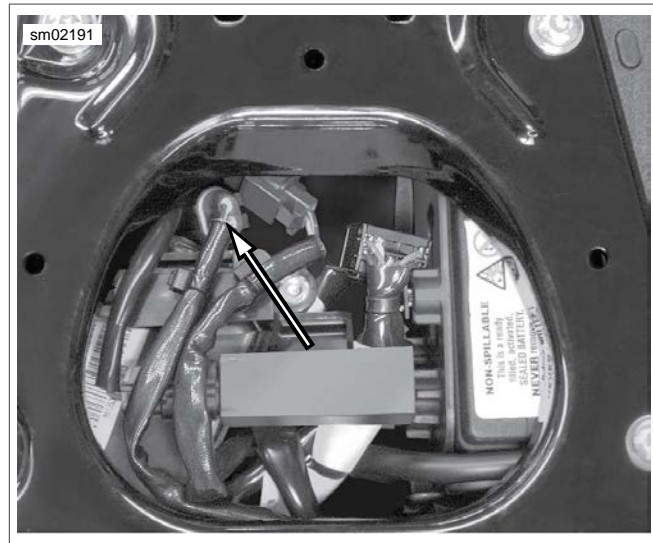
Figure 4-65. Rear O2 Connector and Harness
