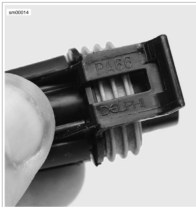
Figure A-10. Delphi Connector: Socket Housing Latch
