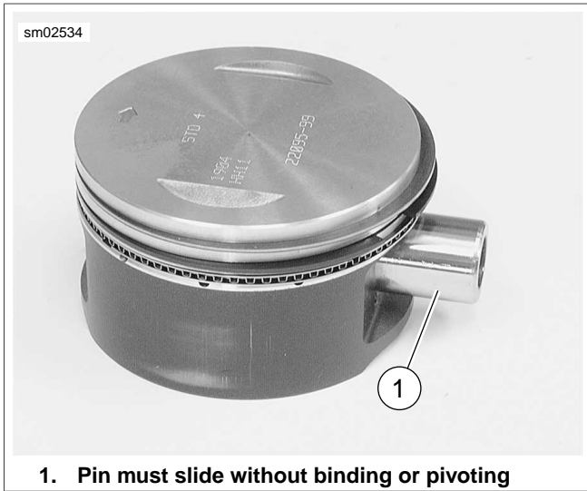
Figure 3-101. Piston Pin Clearance
