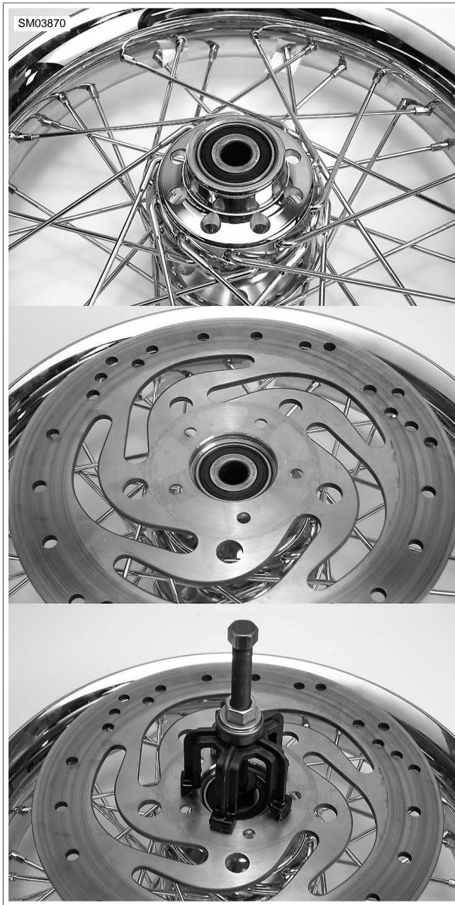
Figure 2-15. Brake Disk as Puller Aid
