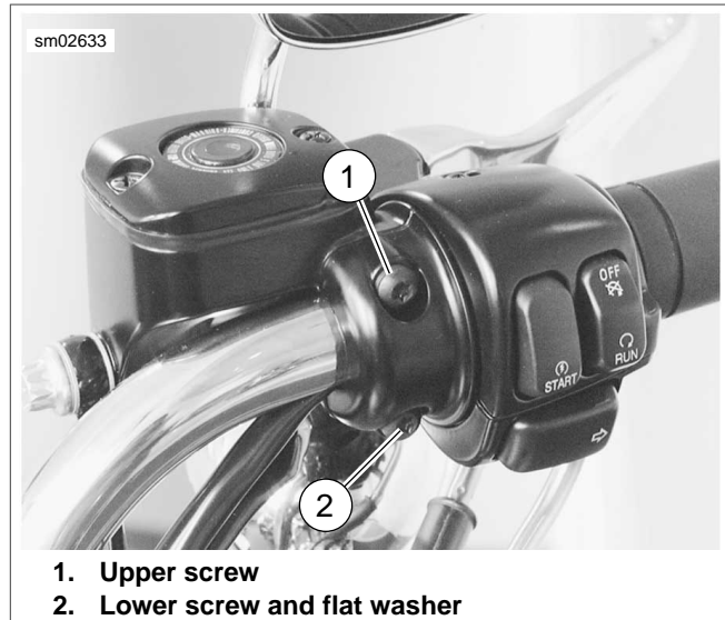
Figure 7-90. Handlebar Switch Clamp Screws
