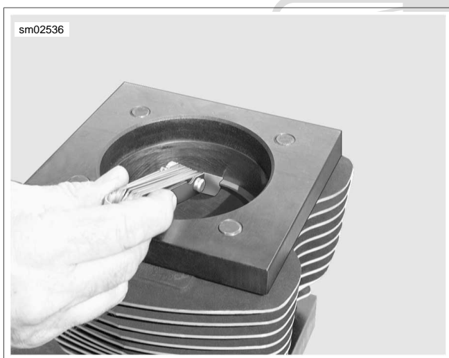
Figure 3-104. Measuring Ring Gap
