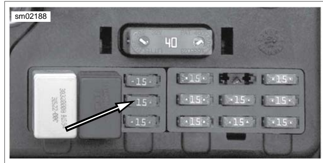
Figure 4-13. Fuel Pump Fuse
