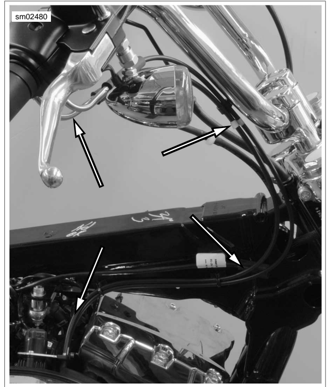
Figure 2-96. Throttle Cable Routing: FXDF (Typical)
