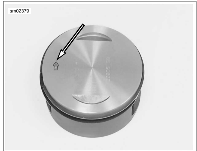
Figure 3-25. Piston Installation Arrow
