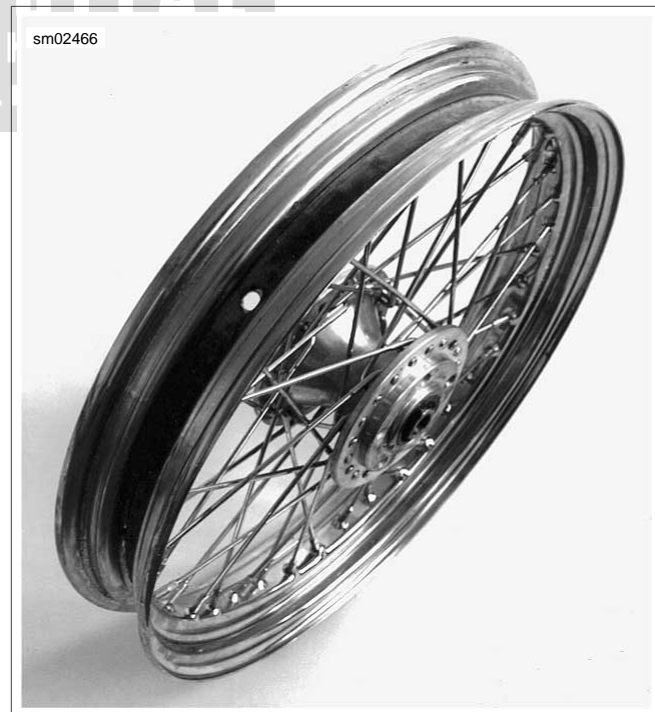
Figure 2-80. Installing Rim Strip
