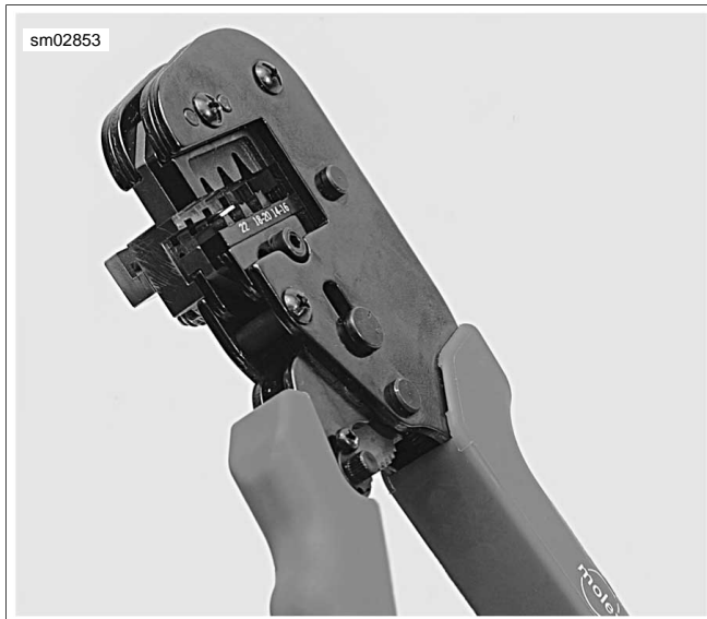
Figure A-30. Open Electrical Crimp Tool (HD-48119) at 45 Degrees
