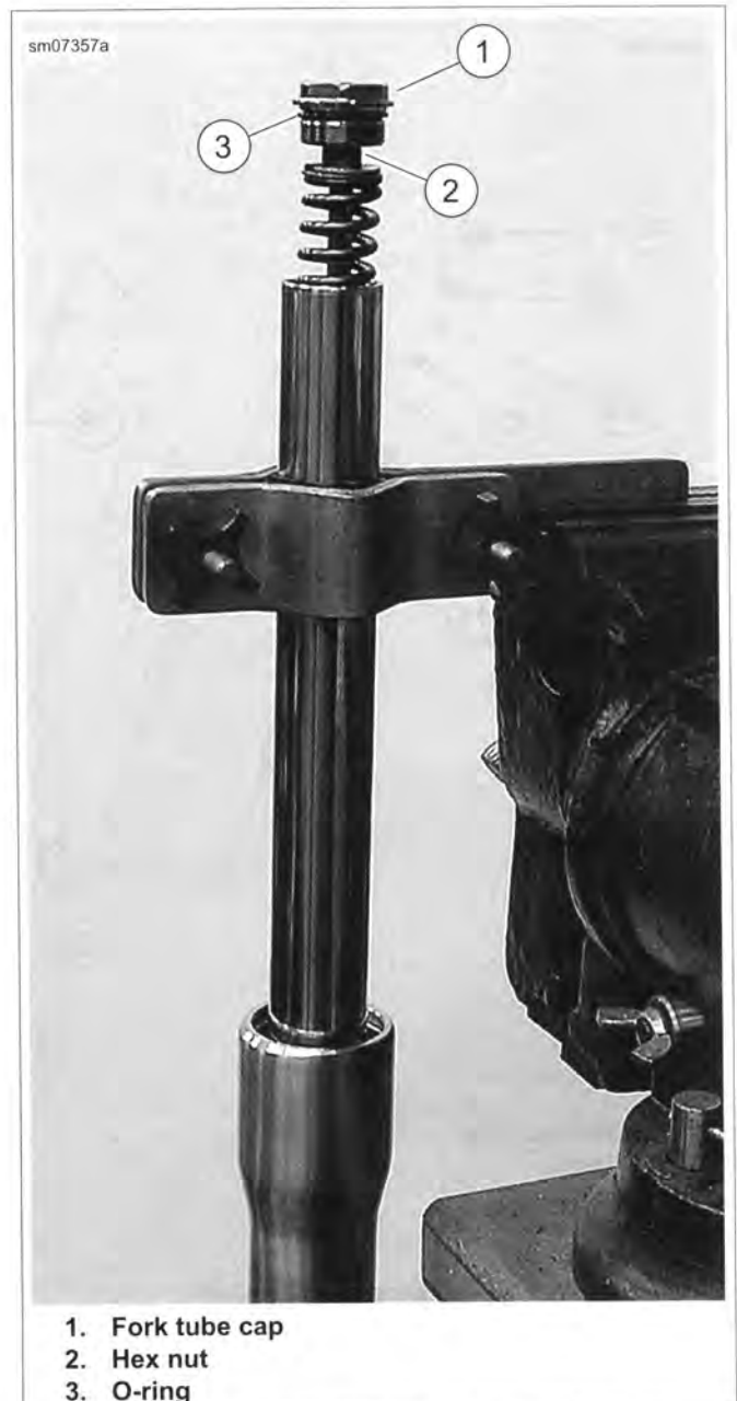
Figure 2-93. Install Fork Tube Into Fork Holder
