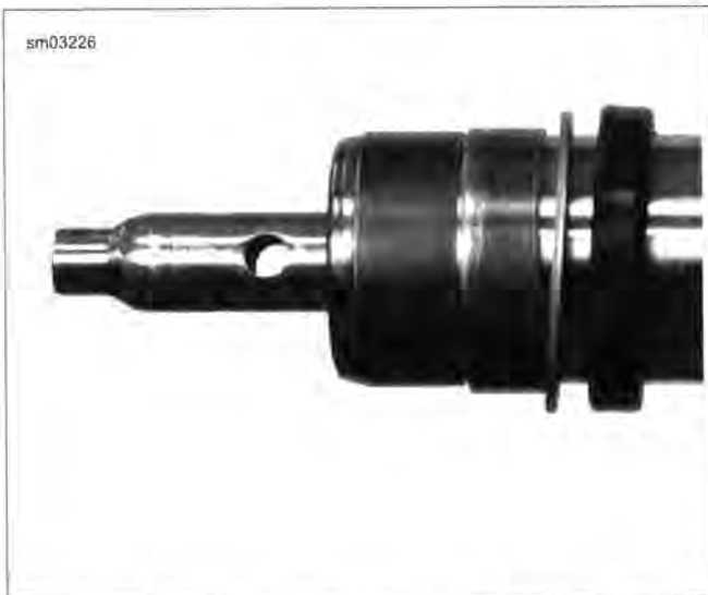
Figure 2-100. Seat Pipe Centered in Fork Tube
