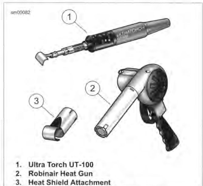
Figure 7-103. Radiant Heating Devices
