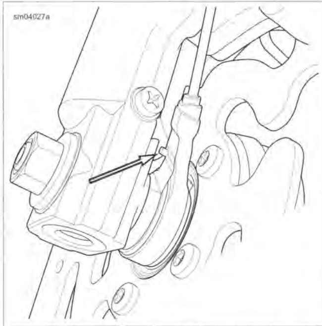
Figure 7-77. Front Wheel Speed Sensor Index Pin (ABS Models)
