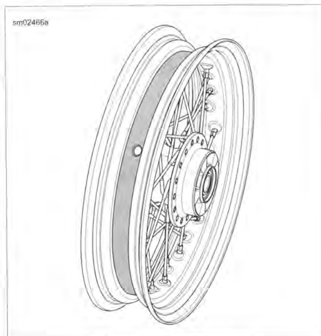
Figure 2-82. Installed Rim Strip
