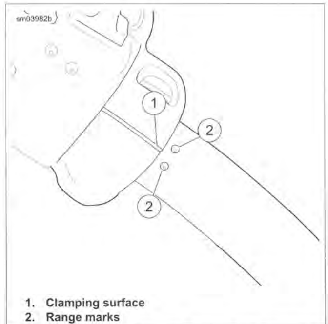
Figure 7-106. Left Hand Control Assembly to Handlebar Alignment: FXDWG Models
