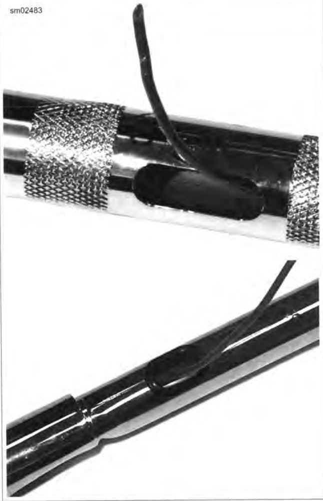
Figure 2-128. Wire Leader in Handlebar (Handlebar Removed from Motorcycle): Typical
