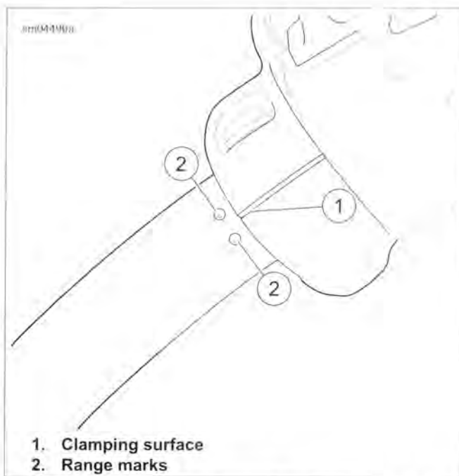
Figure 7-110. Right Hand Control Assembly to Handlebar Alignment: FXDWG Models
