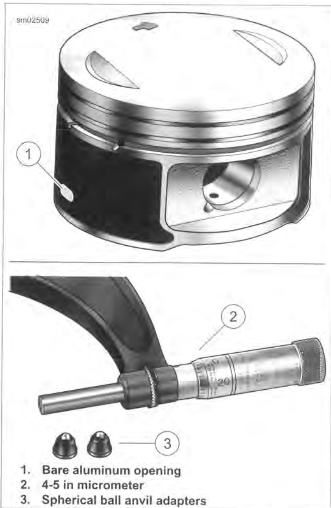
Figure 3-56. Measuring Running Clearance of Piston
