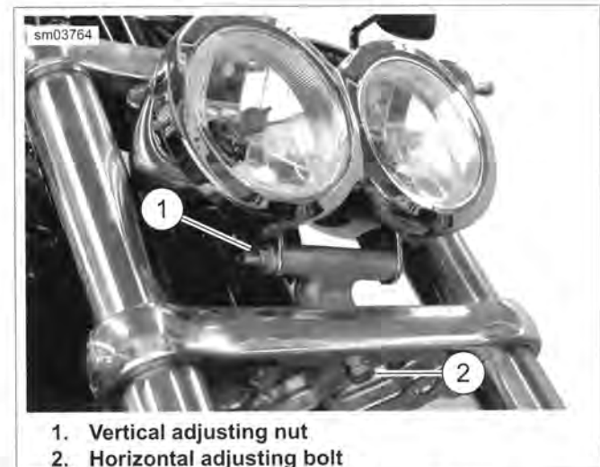
Figure 1-44. Headlamp Adjustments: Dual Bulb
