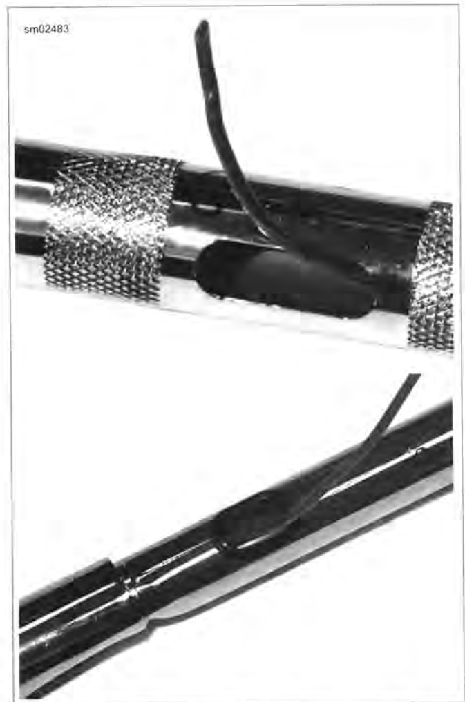
Figure 2-130. Wire Leader in Handlebar (Handlebar Removed from Motorcycle): Typical
