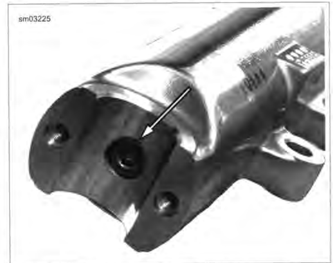
Figure 2-90. Seat Pipe Screw (right fork assembly)
