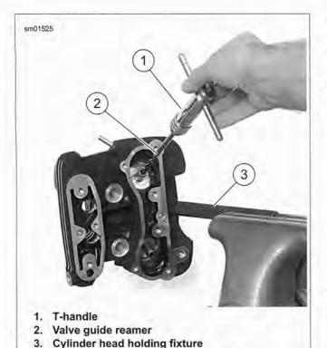
Figure 3-63. Reaming Valve Guide Bore
