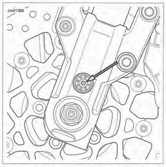
Figure 1-69. Spring Preload Adjuster: XR 1200X
