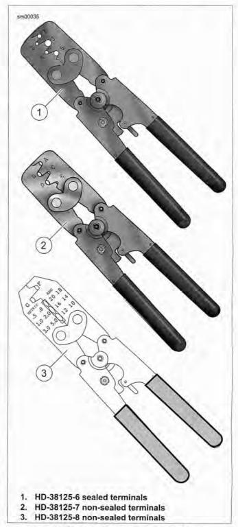
Figure A-13. Metri-Pack Terminal Crimp Tools
