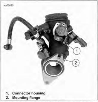
Figure 4-24. Throttle Position (TP) Sensor Installation: XR 1200X
