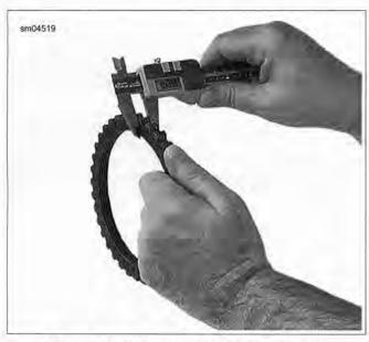
Figure 5-12. Measuring Clutch Friction Plates
