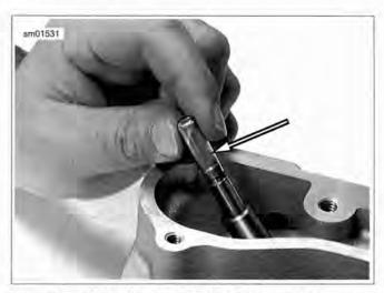
Figure 3-68. Valve Guide Seal Protector Sleeve
