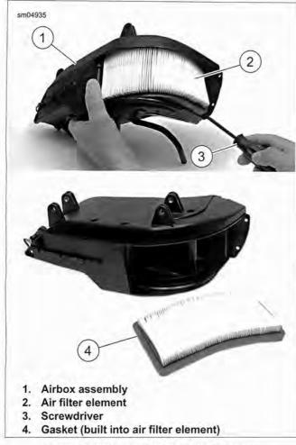
Figure 1-80. Removing Air Filter Element
