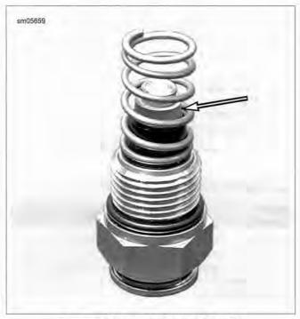
Figure 3-139. Thermostat: XR 1200X
