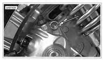
Figure 1-23. Brake Pad Pin (plug removed)
