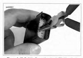
Figure A-45. Pull Up Secondary Lock (Pin Housing)
