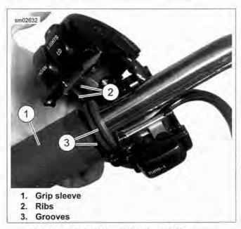
Figure 6-153. Left Handlebar Switch Housings
