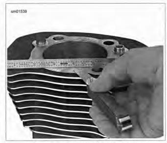
Figure 3-73. Checking Gasket Surfaces
