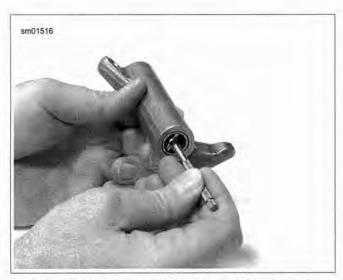
Figure 3-55. Measuring Rocker Arm Bushing Inner Diameter
