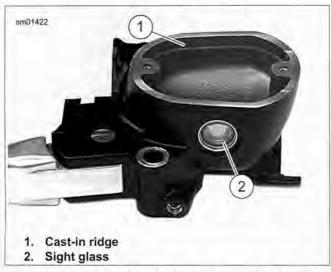
Figure 1-19. Filling Front Master Cylinder Reservoir (typical)
