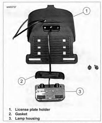
Figure 6-70. Lamp Housing Separated from License Plate Holder: XL 883N, XL 1200N/X (HDI)
