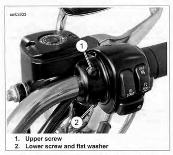
Figure 6-148. Handlebar Switch Clamp Screws
