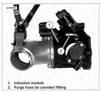
Figure 4-88. Emissions Hose Routing at Induction Module
