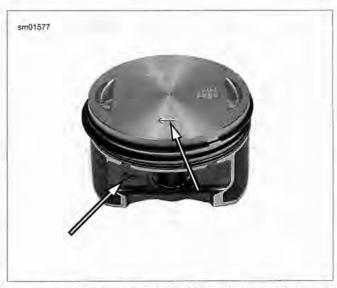
Figure 3-88. Arrows on Piston Must Point Toward Front of Engine (typical; XL shown)
