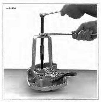
Figure 3-112. Removing Cam Bushing from Gearcase Cover
