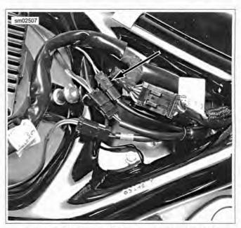
Figure 6-62. License Plate Lamp Connector [40]
