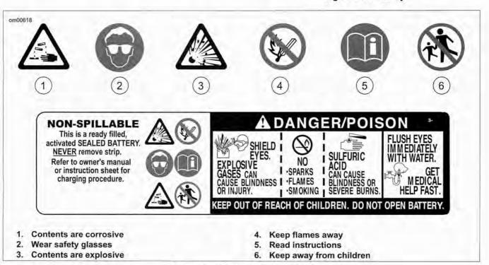
Figure 1-59, Battery Warning Label
