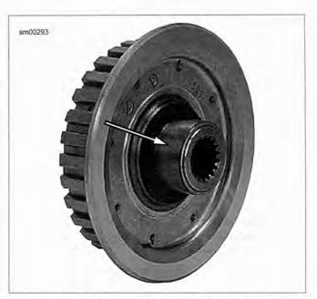
Figure 5-27. Clutch Hub Bearing Race
