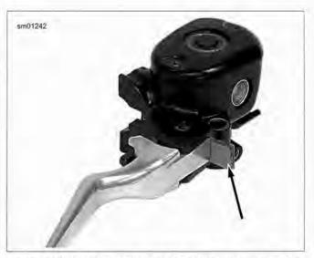
Figure 2-44. Install 5/32 in (4 mm) Cardboard Insert Before Installing Master Cylinder Assembly
