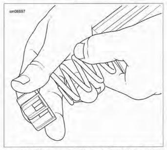
Figure 2-150. Remove the Upper Spring Collar and the Spring
