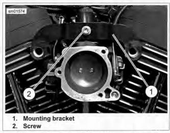
Figure 4-30. Induction Module Mounting Bracket
