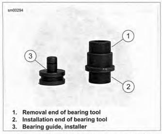
Figure 5-28. Clutch Shell Bearing Remover/Installer
