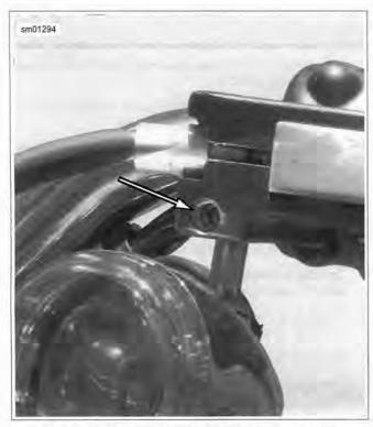
Figure 6-75. Turn Signal Ball Stud Allen Screw
