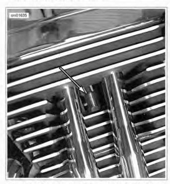
Figure 4-25. Engine Temperature (ET) Sensor Location
