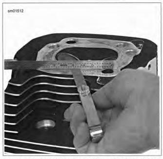
Figure 3-52. Gasket Surface: Flat Within 0.006 in (0.152 mm)
