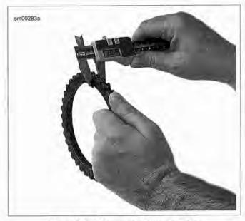
Figure 5-22. Measuring Friction Plates
