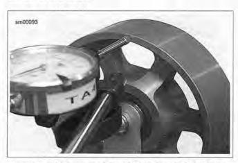
Figure 1-46. Measuring Lateral Side Play on Idler Pulley
