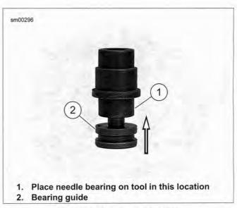
Figure 5-30. Bearing Installer
