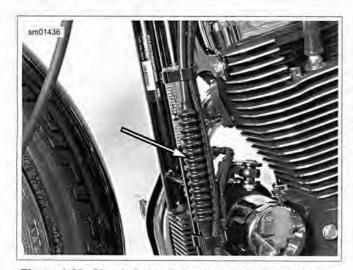
Figure 1-39, Clutch Cable Adjuster Location: XL Models
