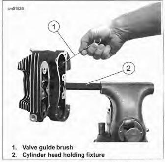
Figure 3-64. Scrubbing Valve Guide Bore
