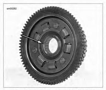
Figure 5-26. New Needle Bearing in Clutch Shell
