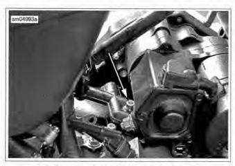
Figure 3-30. Return Oil Manifold Fastener
