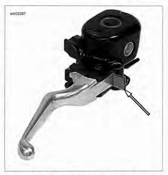
Figure 6-139. Install Cardboard Insert
