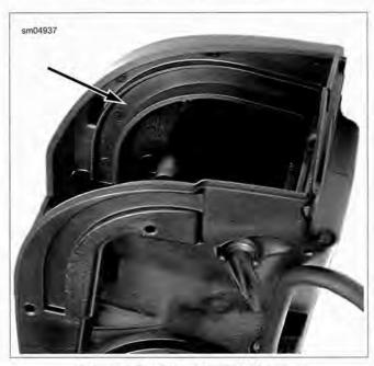
Figure 1-81. Filter Element Channel
