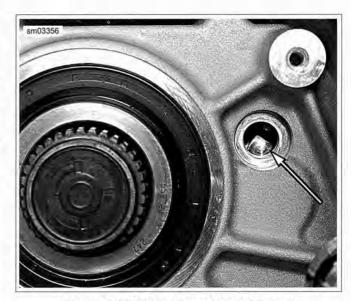
Figure 5-47. Shifter Drum Neutral Detent
