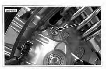
Figure 2-90. Brake Pad Pin (plug removed)
