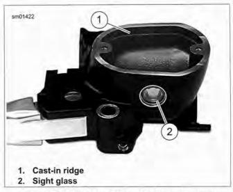
Figure 1-29. Filling Front Master Cylinder Reservoir (typical)
