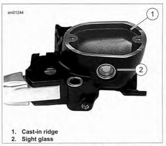
Figure 2-63. Filling Front Master Cylinder Reservoir
