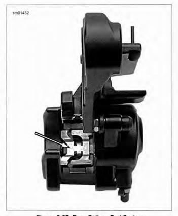
Figure 2-97. Rear Caliper Pad Spring
