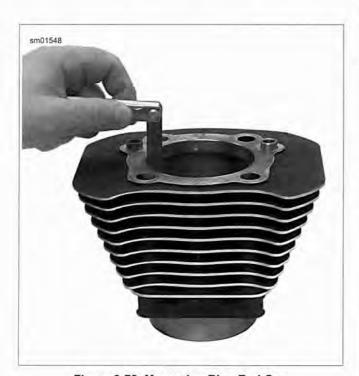
Figure 3-78. Measuring Ring End Gap
