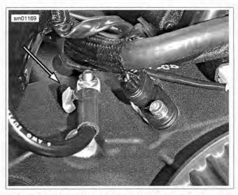
Figure 6-25. Negative Battery Cable Stop on Crankcase (typical)
