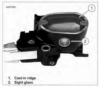
Figure 2-48. Filling Front Master Cylinder Reservoir
