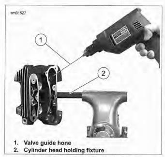
Figure 3-65. Honing Valve Guide Bore
