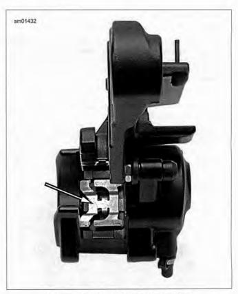
Figure 1-21. Rear Caliper Pad Spring
