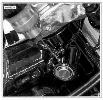
Figure 2-234. Drilling Lock Pin
