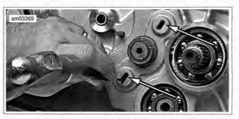
Figure 5-56. Slots For Removing Shifter Fork Shafts
