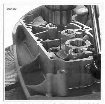
Figure 3-115. Drilling Pinion Bushing Dowel Pin Hole in Gearcase Cover
