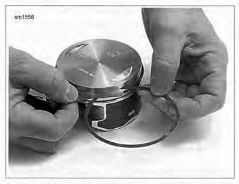
Figure 3-82. Measuring Ring Clearance in Groove (typical)
