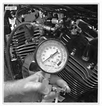
Figure 4-80. Fuel Pressure Gauge Installed: All Models
