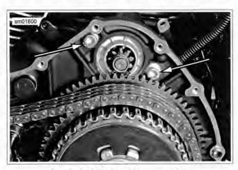
Figure 6-28. Starter Mounting Bolts
