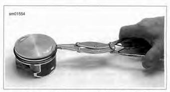
Figure 3-80. Installing Piston Rings (typical)
