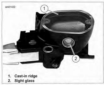
Figure 2-122. Filling Front Master Cylinder Reservoir (typical)
