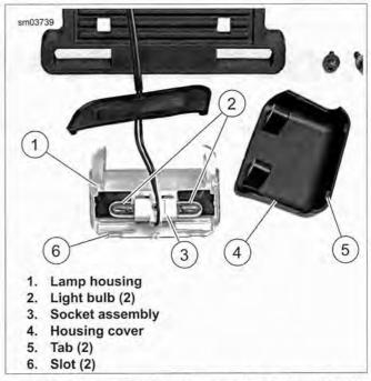
Figure 6-72. Replacing License Plate Light Bulbs: XL 883N, XL 1200N/X (HDI)
