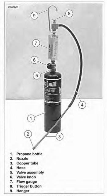
Figure 4-81. Leak Tester
