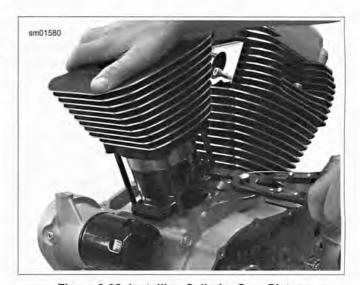
Figure 3-92. Installing Cylinder Over Piston
