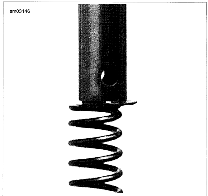
Figure 2-156. Remove Collar, Washer and Spring
