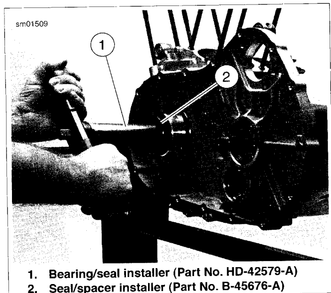
Figure 3-89. Install Bearing Seal/Spacer
