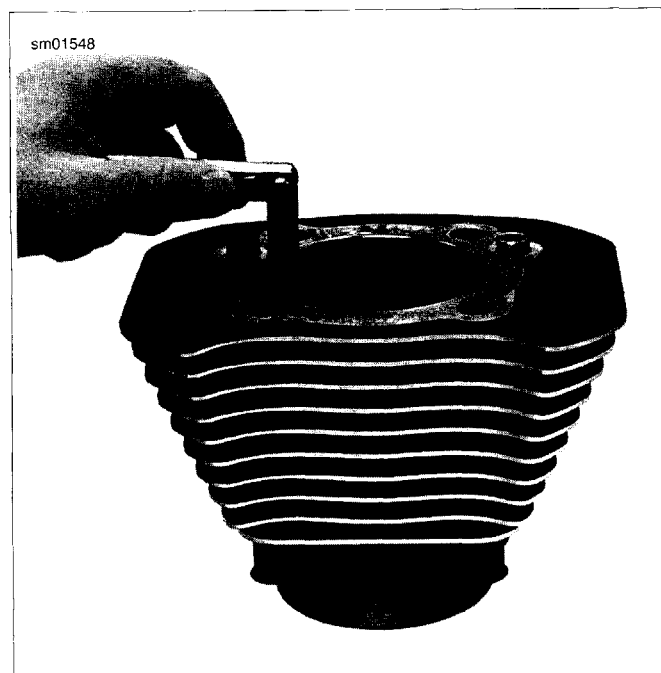
Figure 3-141. Measuring Ring End Gap
