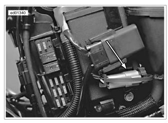
Figure 2-24. Data Link Connector [91A] (Behind Left Side Cover)
