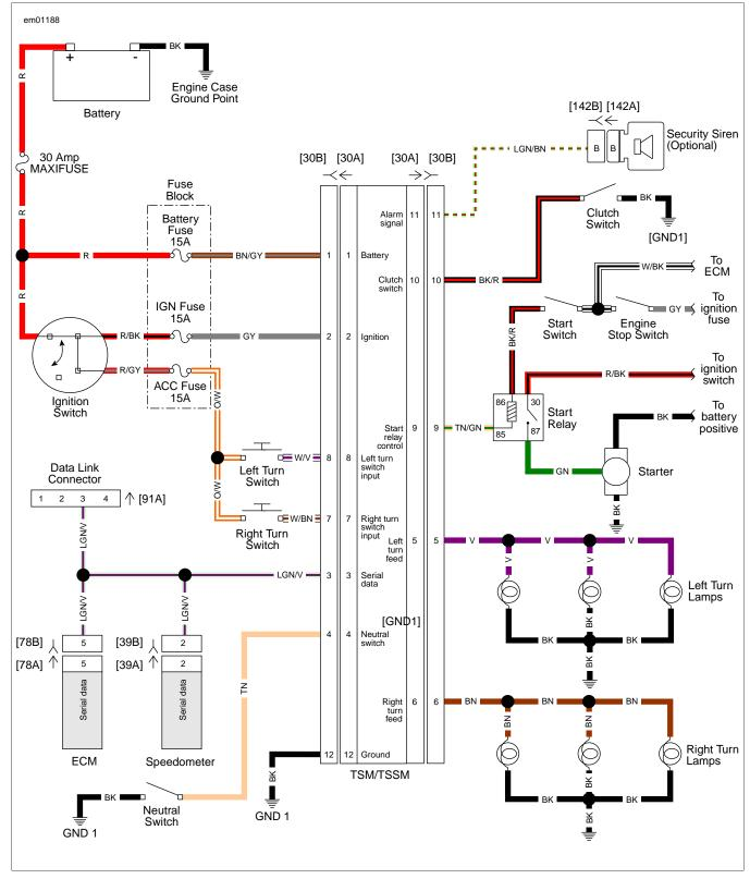
Figure E-3. Simplified TSM/TSSM Wiring
