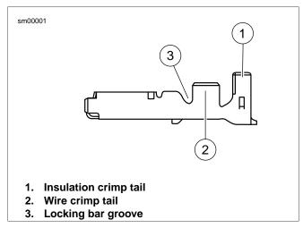
Figure A-7. AMP Multilock Connector: Socket Terminal
