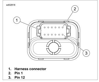
Figure E-14. TSM/TSSM Connector [30A]
