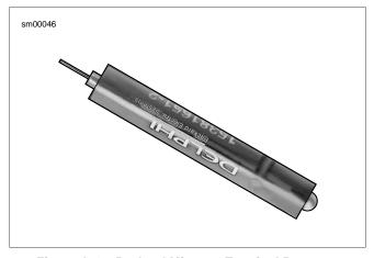
Figure A-43. Packard Micro 64 Terminal Remover (HD-45928)
