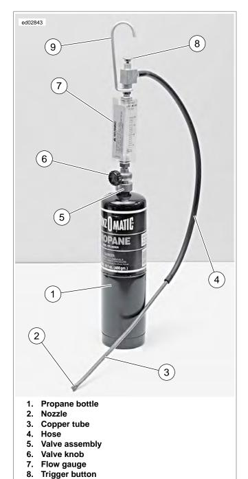
Figure 4-12. Leak Tester
