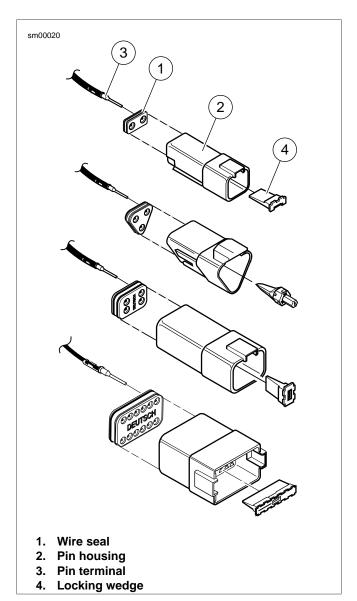
Figure A-18. Deutsch Connector: 2, 3, 4 and 12-Place Pin Housings
