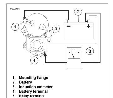
Figure 1-8. Free Running Current Draw Test
