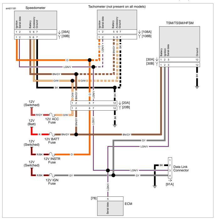
Figure 3-11. Initial Diagnostic Check
