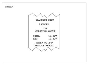
Figure 1-17. Charging System Test Results Printout
