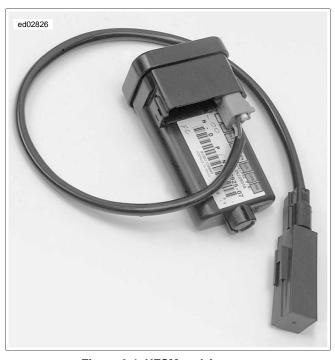
Figure 3-1. HFSM and Antenna
