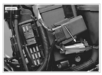
Figure 4-52. Data Link Connector [91A]
