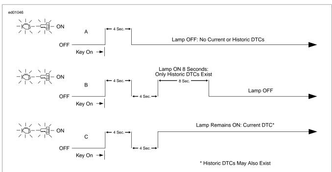
Figure 2-3. Check Engine and Security Lamp Operation
