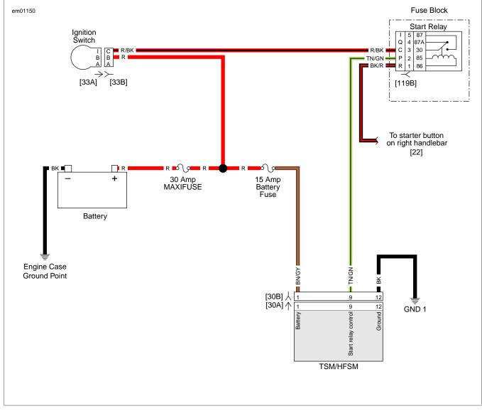
Figure 3-26. Starter TSM/HFSM Circuits
