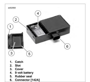
Figure E-32. Siren Battery Compartment (Late Style Siren)
