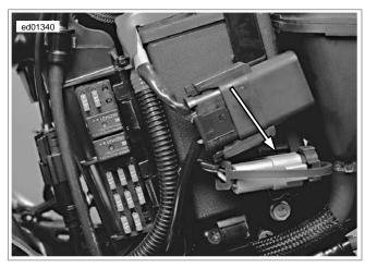
Figure E-28. Data Link Connector [91A]
