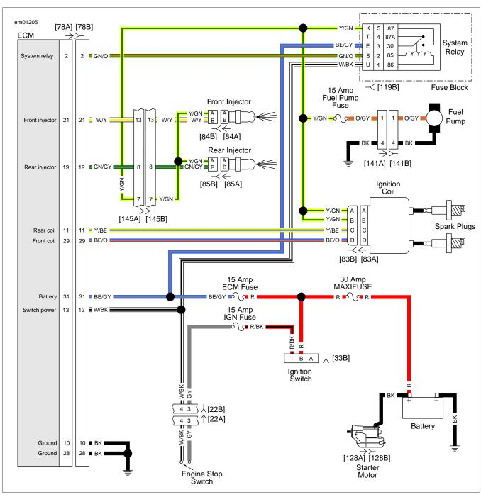
Figure 4-35. Ignition Coil Circuit Diagram
