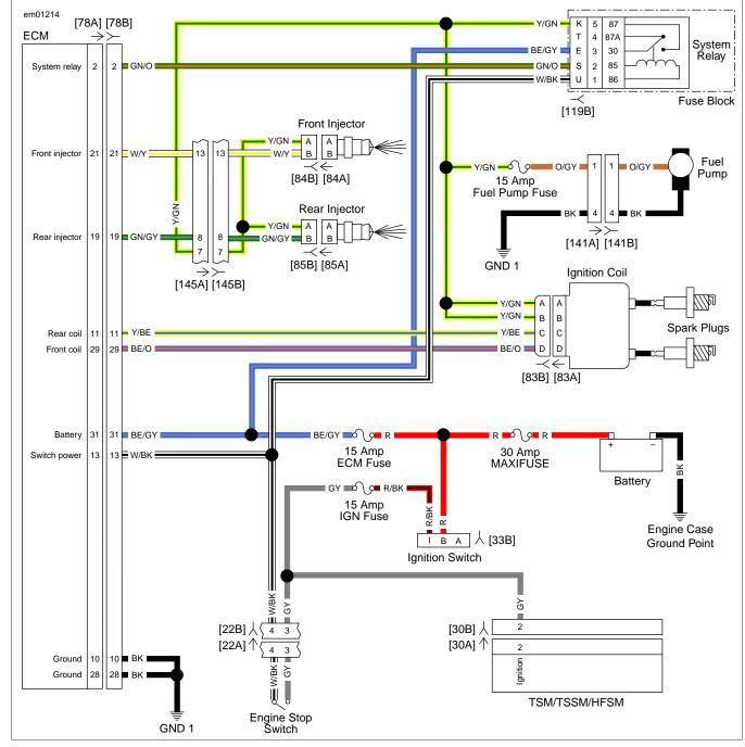
Figure 4-57. Ignition Coil Circuit
