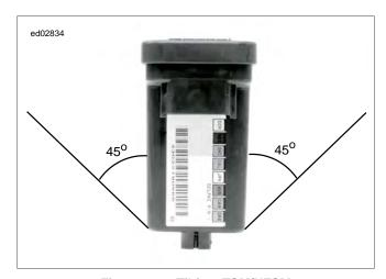
Figure 3-22. Tilting: TSM/HFSM
