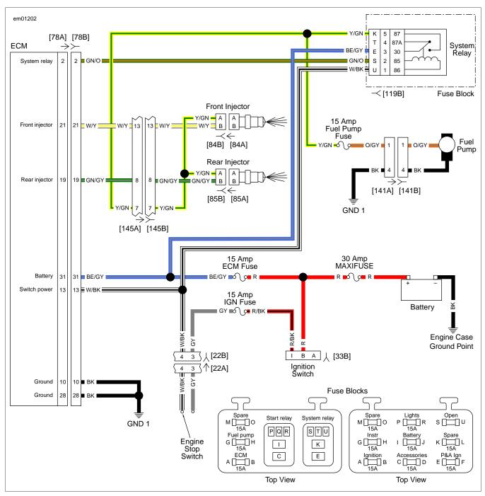
Figure 4-23. Fuel Pump Circuit
