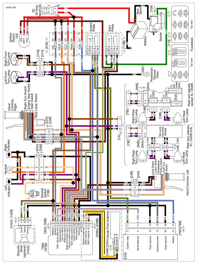
Figure 3-21. Turn Signal Circuit
