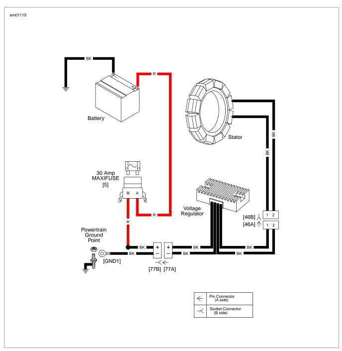
Figure 1-14. Charging System Circuit
