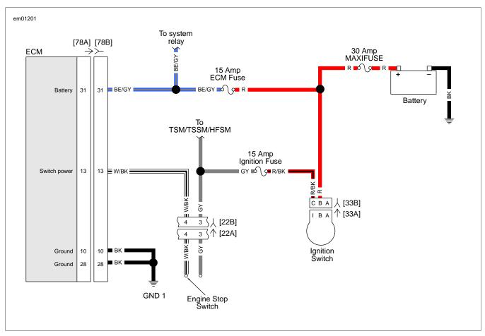
Figure 4-18. ECM Power Circuit Diagram
