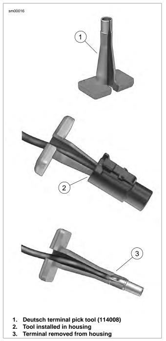
Figure A-12. Deutsch 1-Place Connector: Remove Socket/Pin Housing
