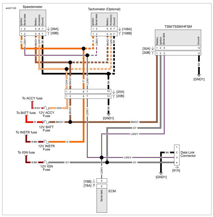
Figure 4-20. Serial Data Circuit
