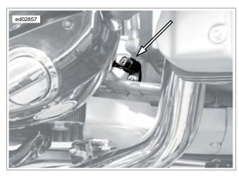
Figure 4-48. Vehicle Speed Sensor and Connector
