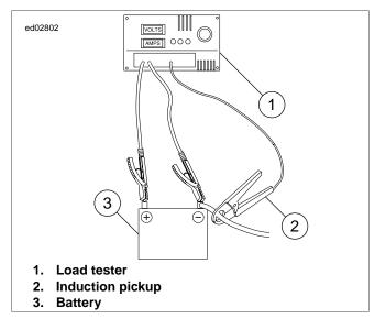
Figure 1-16. Check Current Draw (Ignition Switch On)
