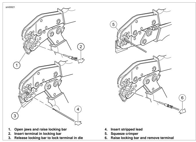
Figure A-19. Crimping a Deutsch Standard Terminal
