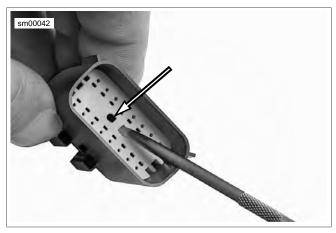
Figure A-37. Molex Connector: Secondary Lock D-Holes (Pin Housing)
