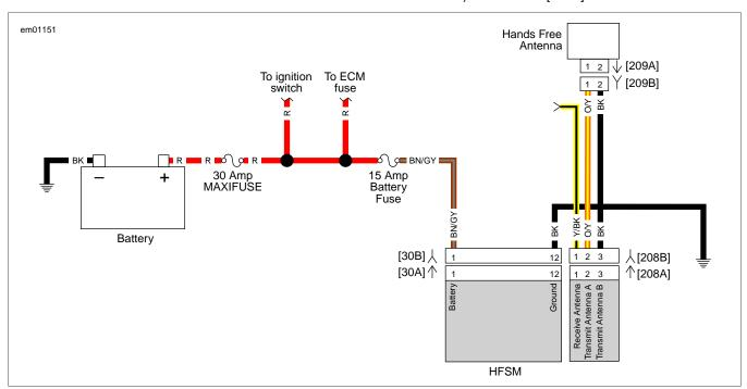
Figure 3-27. Security Antenna Circuit
