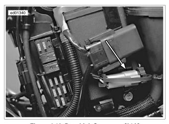
Figure 4-19. Data Link Connector [91A]
