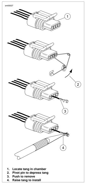
Figure A-25. 150 Metri-Pack Connector: Pull-to-Seat
