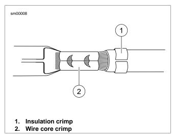
Figure A-9. AMP Multilock Connector: Terminal Crimp
