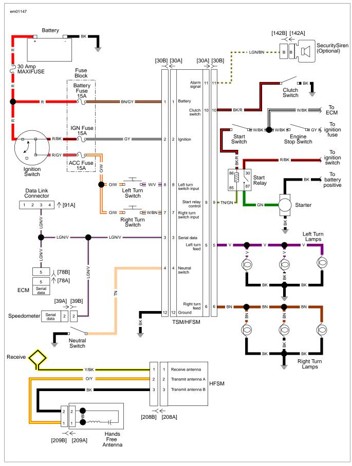
Figure 3-5. Simplified TSM/HFSM Wiring
