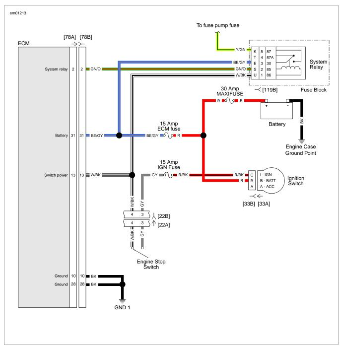
Figure 4-51. Ignition Coil Circuit
