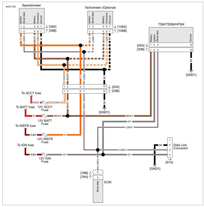
Figure 4-63. Serial Data Circuit
