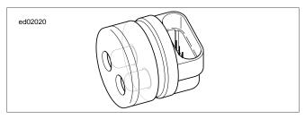
Figure 4-30. IAC Test Lamp (Part No. HD-41199-3)
