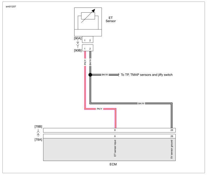
Figure 4-39. ET Sensor Circuit
