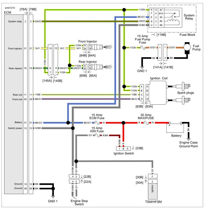
Figure 4-45. Fuel Injector Circuit
