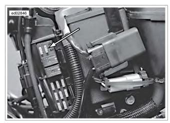
Figure 4-26. Fuel Pump Fuse
