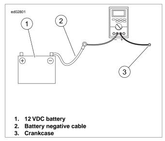
Figure 1-15. Milliampere Draw Test (Ignition turned to OFF)
