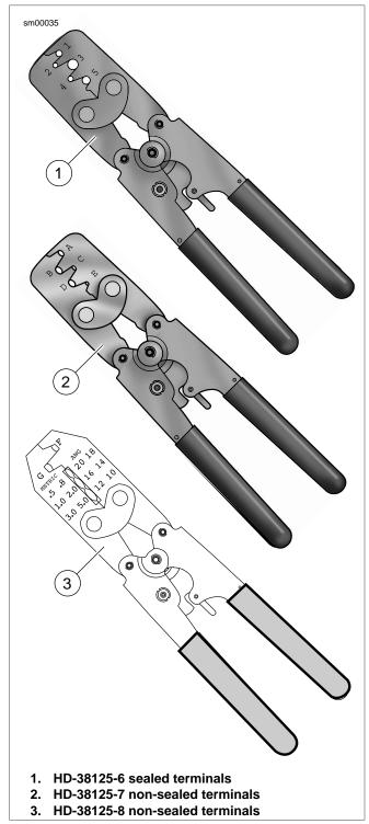
Figure A-33. Metri-Pack Terminal Crimp Tools
