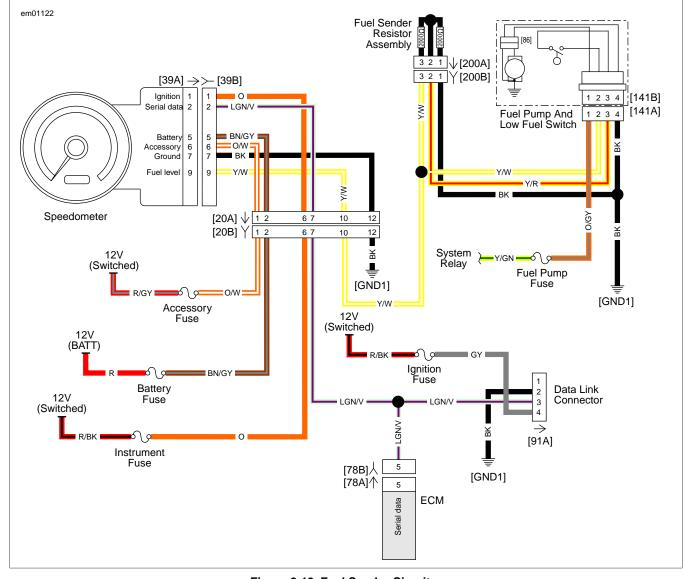
Figure 2-13. Fuel Sender Circuitry
