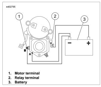
Figure 1-9. Pull-In Test
