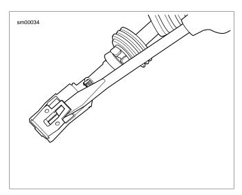
Figure A-32. Delphi Maxi-Fuse Housing: Bend Tang
