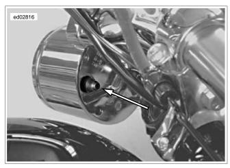
Figure 2-6. Trip Odometer Reset Switch (Typical)
