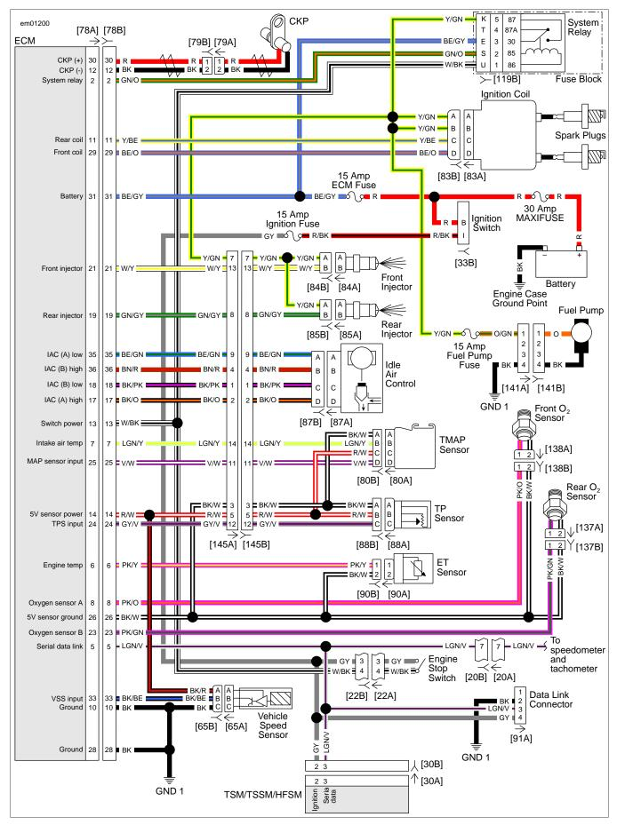
Figure 4-2. EFI System Circuit
