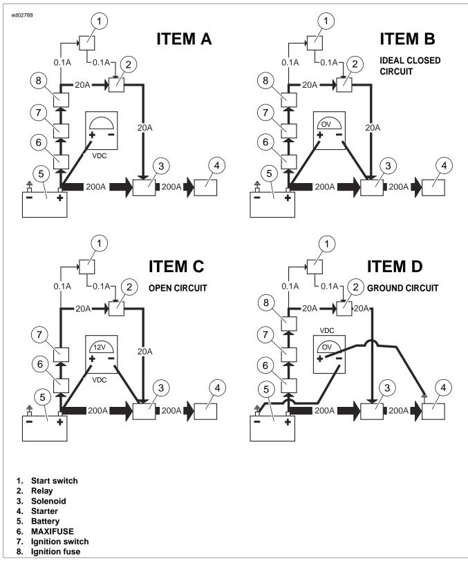
Figure 1-3. Typical Circuitry. Refer to wiring diagrams for more information.
