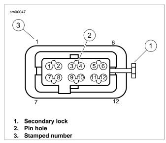
Figure A-45. Packard Micro 64 Connector: Housing
