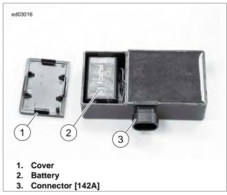
Figure 3-33. Battery Compartment (Early Style Siren)
