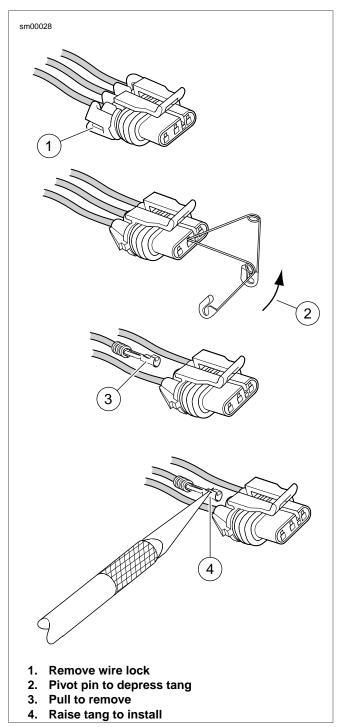
Figure A-26. 150 Metri-Pack Connector: Push-to-Seat
