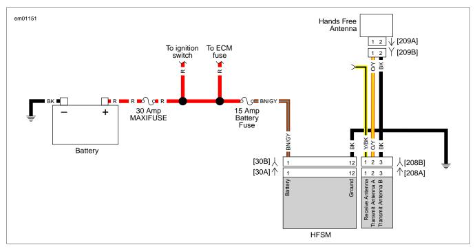
Figure 3-20. Antenna Circuit: HFSM
