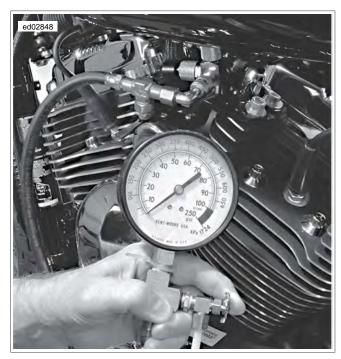
Figure 4-29. Fuel Pressure Gauge Installed
