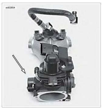
Figure 4-40. Throttle Position (TP) Sensor Location
