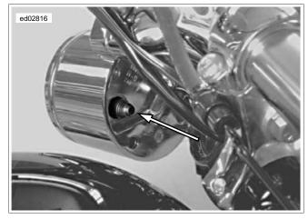
Figure 3-12. Trip Odometer Reset Switch (Typical)
