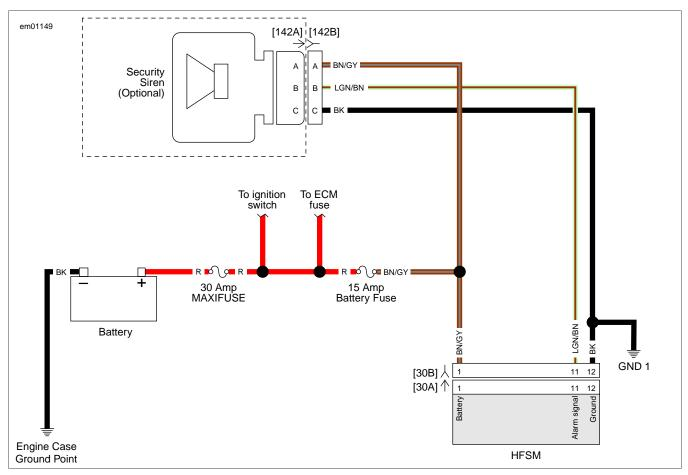
Figure 3-24. Smart Siren Circuit
