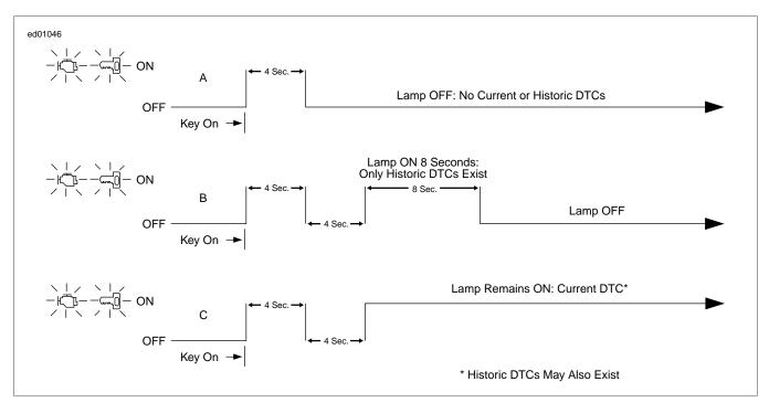
Figure E-9. Security Lamp Operation
