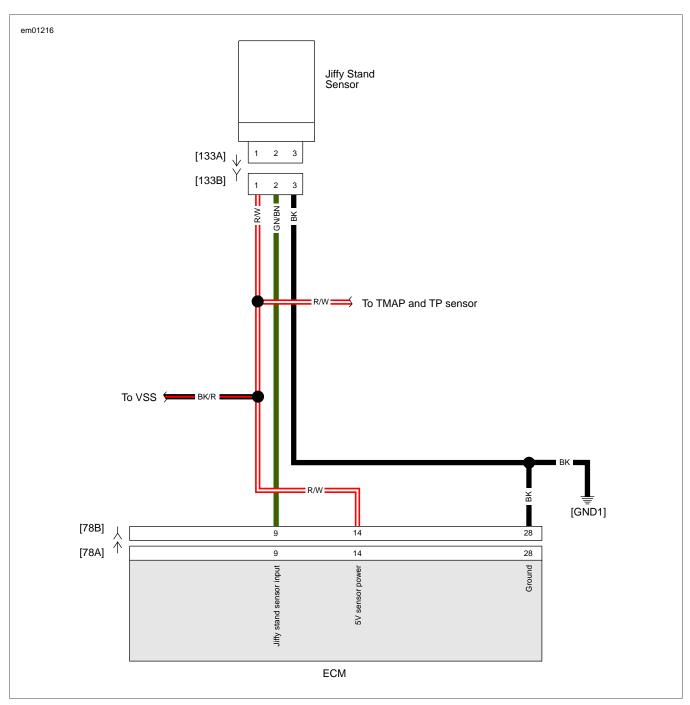
Figure 4-60. Jiffy Stand Sensor Circuit
