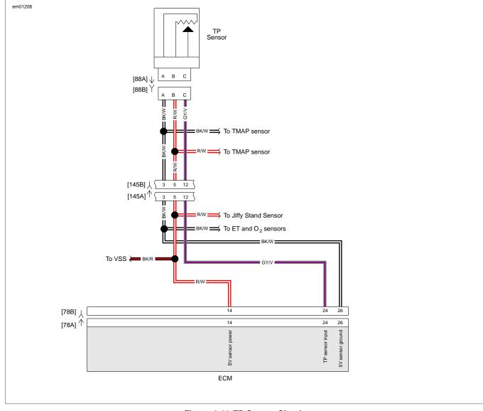
Figure 4-41. TP Sensor Circuit
