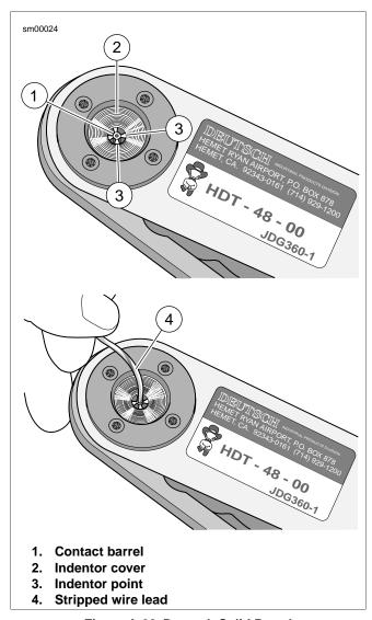
Figure A-22. Deutsch Solid Barrel
