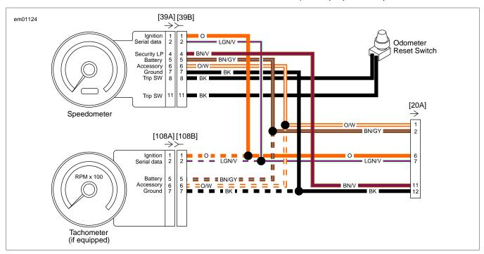
Figure 2-8. Speedometer/Tachometer Circuitry
