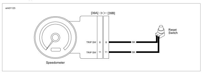
Figure 2-15. Trip Odometer Reset Switch Circuit
