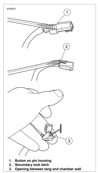
Figure A-29. 480 Metri-Pack Connector: Remove Socket Terminal
