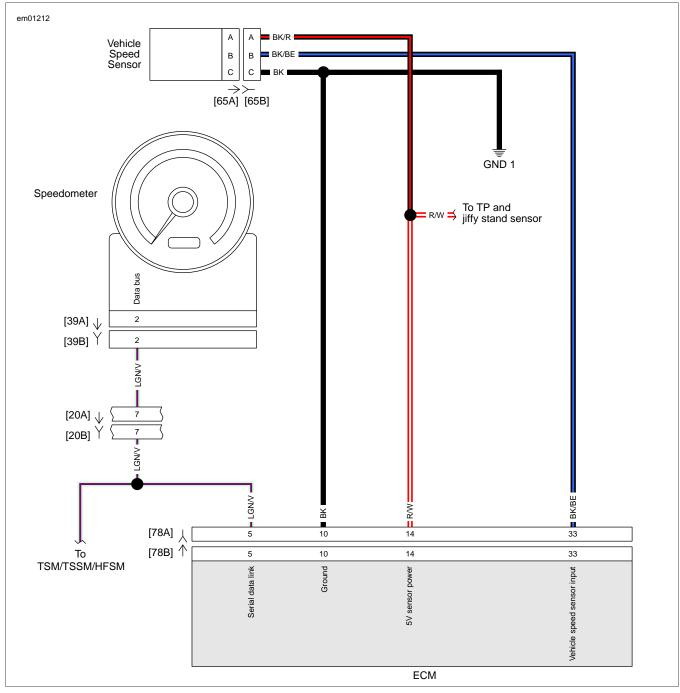
Figure 4-49. Vehicle Speed Sensor
