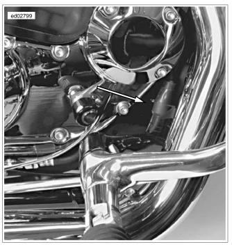
Figure 1-13. Stator Connector [46]
