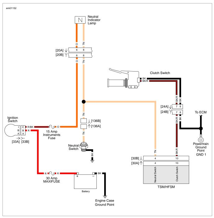
Figure 3-28. Clutch and Neutral Interlock Circuits
