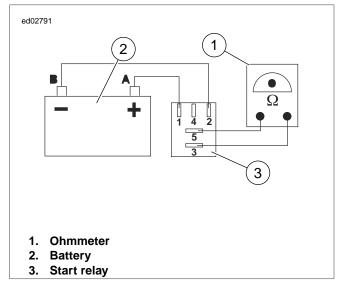
Figure 1-5. Start Relay Test
