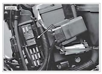
Figure 4-24. System Relay
