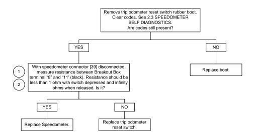
Clear DTCs using speedometer self diagnostics. See 2.3
