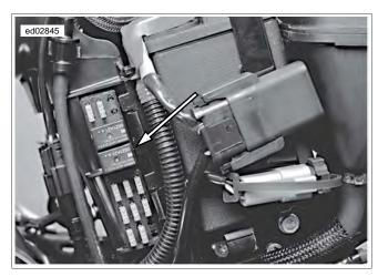
Figure 4-50. System Relay
