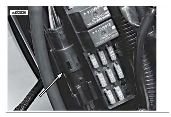
Figure 4-21. Fuel Pump Connector [141]
