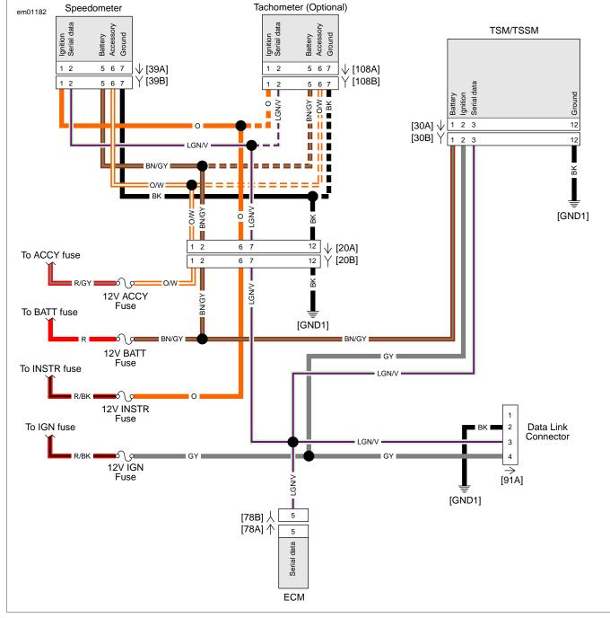
Figure E-27. Serial Data Circuit
