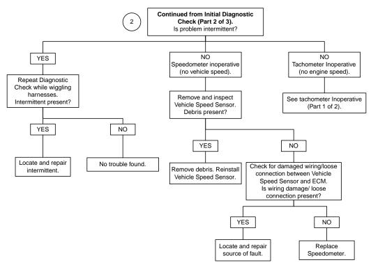
The speedometer is capable of displaying and clearing speedometer, tachometer, TSM/TSSM, and Electronic Control Module (ECM) Diagnostic Trouble Codes (DTCs) (diagnostic mode).
