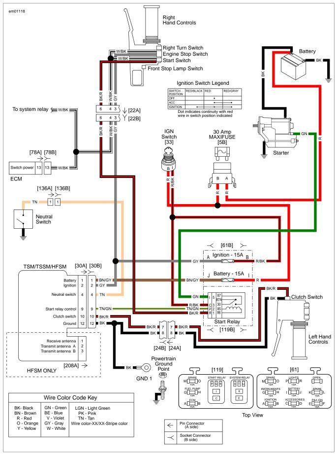
Figure 1-2. Starting Circuit Schematic
