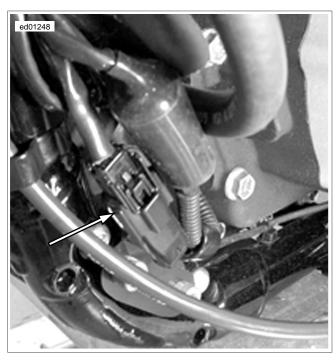
Figure 4-59. Jiffy Stand Sensor Connector
