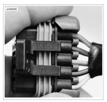
Figure A-27. 280 Metri-Pack Connector (P.E.D.)
