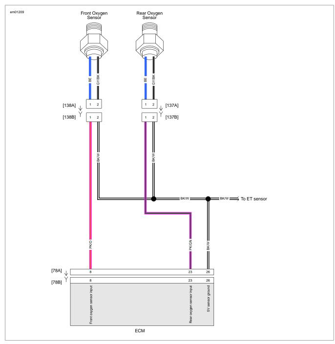
Figure 4-43. Oxygen Sensor
