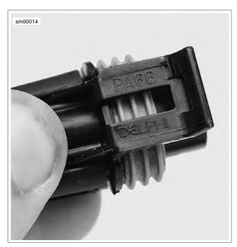
Figure A-10. Delphi Connector: Socket Housing Latch
