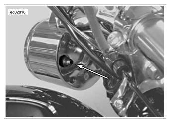
Figure 2-14. Trip Odometer Reset Switch (Typical)
