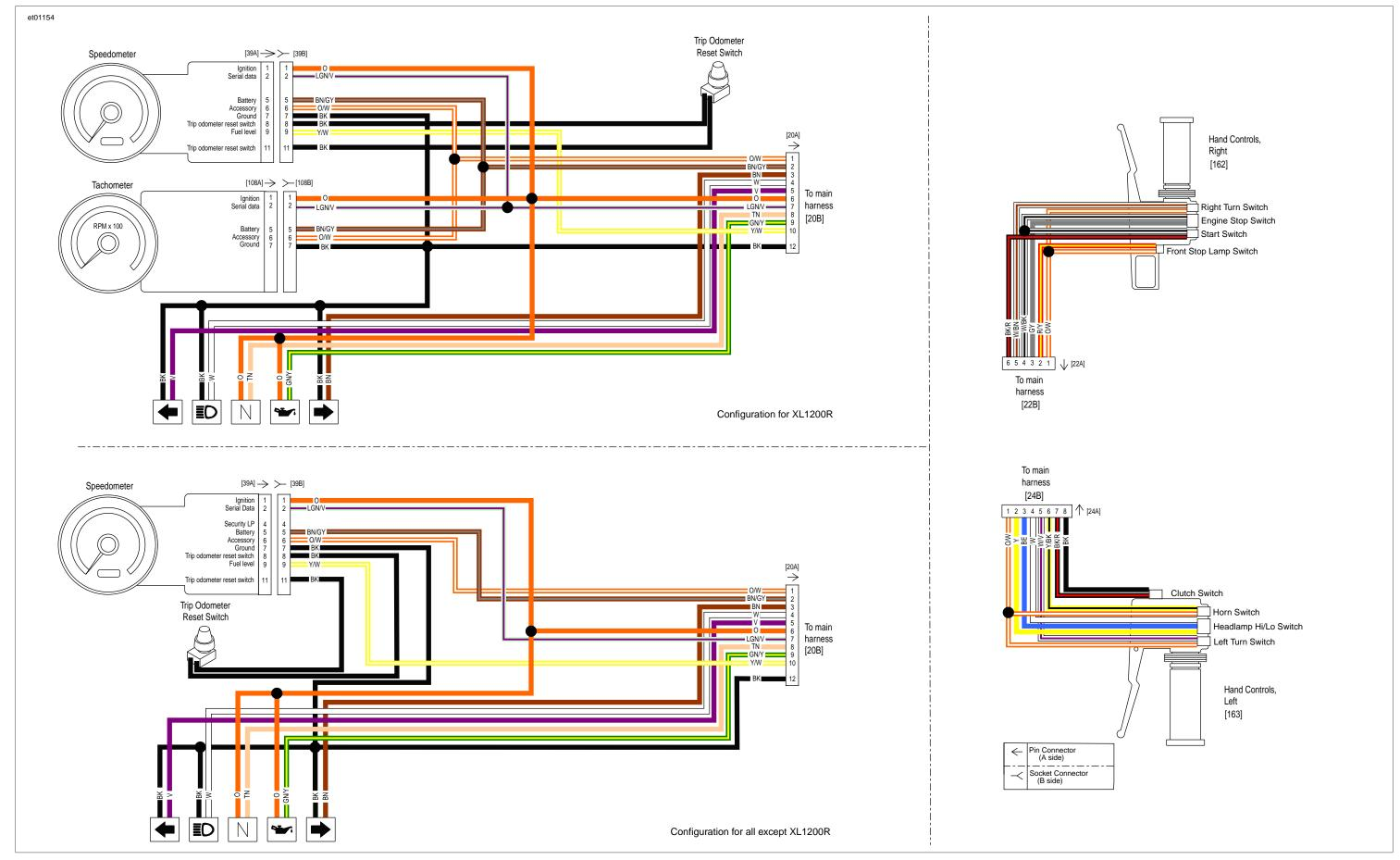
Figure B-3. 2008 SPORTSTER DOM. and INT. MODELS, INDICATOR LAMPS AND CONTROLS
