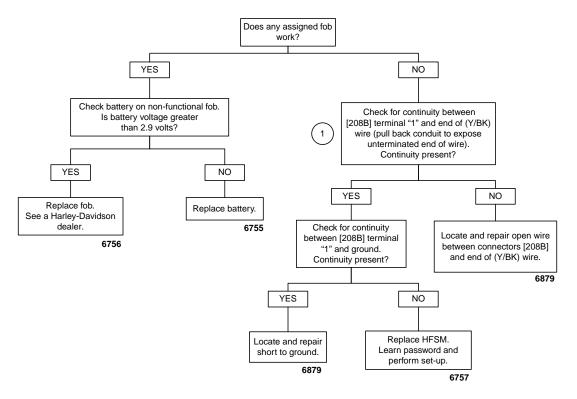
NOTE The fob for the HFSM must be assigned using Digital Technican. Digital Technician can also validate fob operation when connected to the motorcycle.
