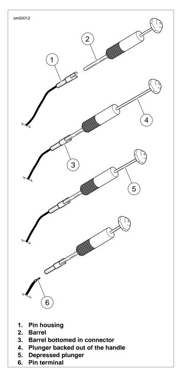
Figure A-2. AMP Pin Terminal Remover (HD-39621-28)
