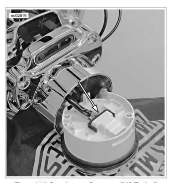
Figure 2-18. Speedometer Connector [39] (Typical)
