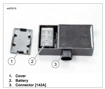
Figure E-31. Battery Compartment (Early Style Siren)
