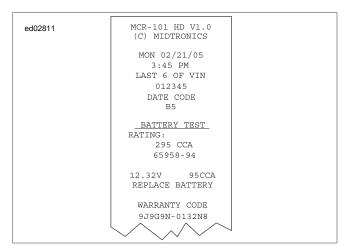
Figure 1-22. Battery Test Results Printout
