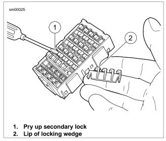
Figure A-23. Fuse Block: Remove Secondary Locks
