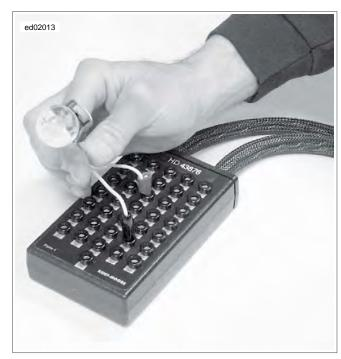
Figure 4-15. Ignition Coil Circuit Test
