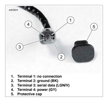
Figure 2-17. Data Link Connector [91A] Terminals
