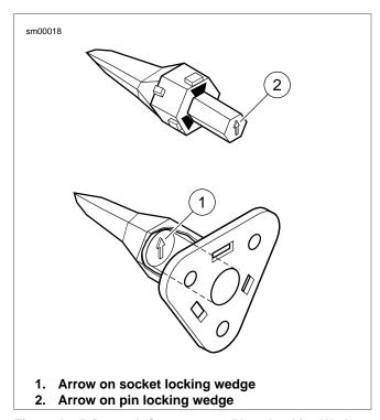
Figure A-15. Deutsch Connector: 3-Place Locking Wedges
