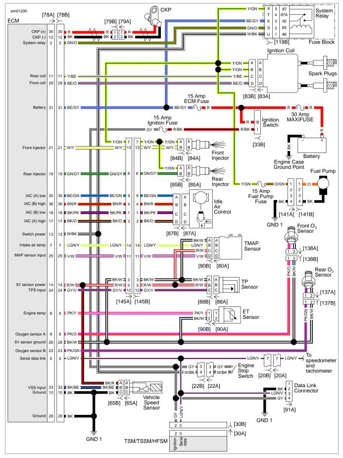
Figure 4-16. EFI Circuit Diagram
