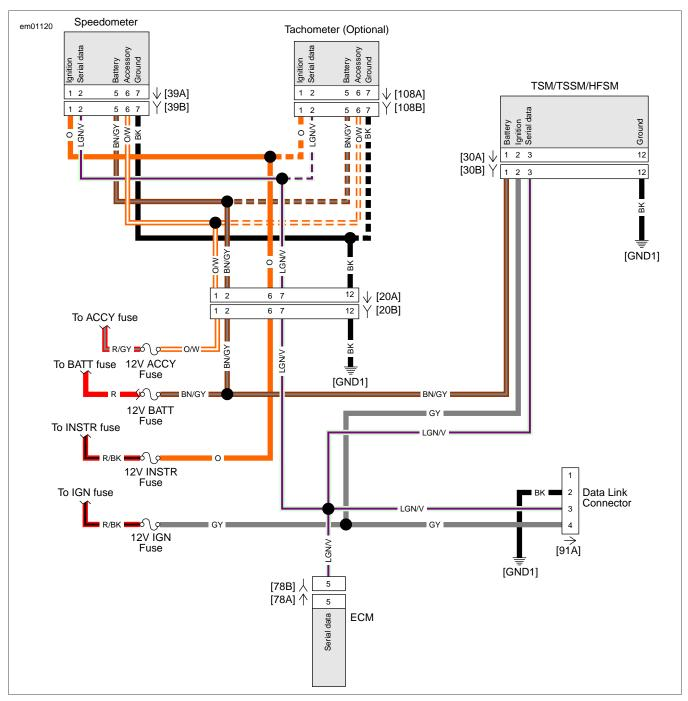
Figure 4-65. Serial Data Circuit
