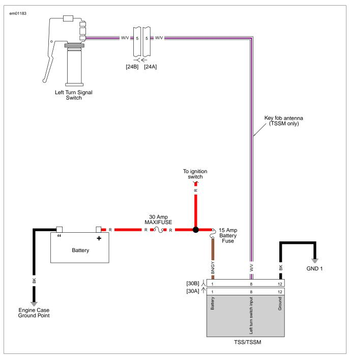
Figure E-17. Antenna Circuit
