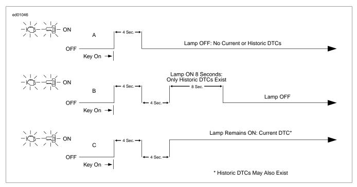
Figure 3-10. Security Lamp Operation
