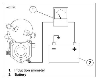
Figure 1-6. Starter Current Draw Test
