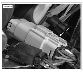
Figure A-35. Molex Connector: Latch
