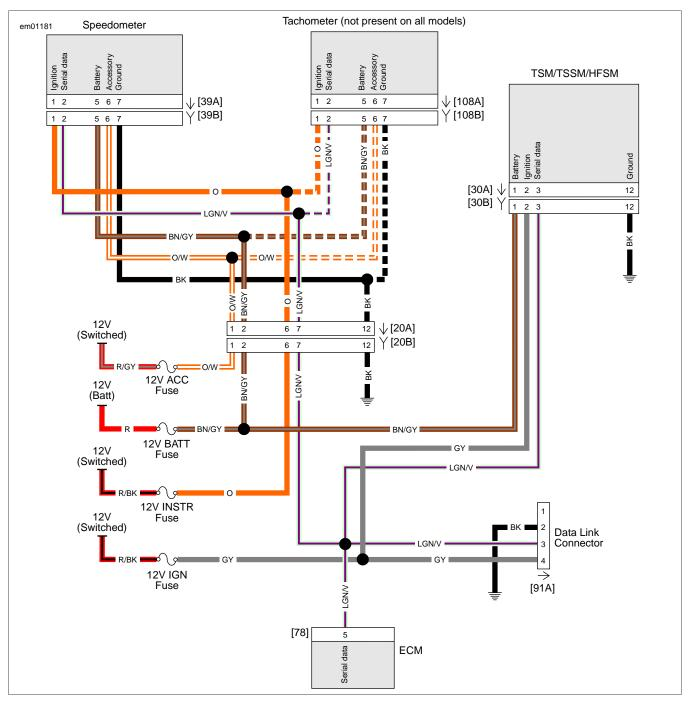
Figure 3-30. Serial Data Circuit
