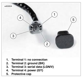
Figure 2-22. Data Link Connector [91A] Terminals
