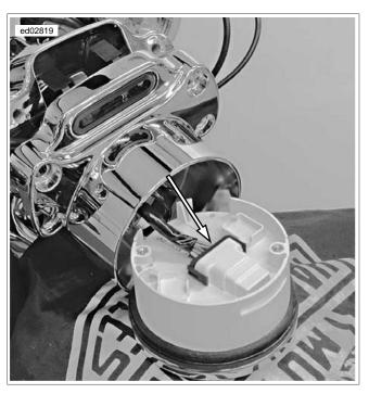
Figure 4-64. Speedometer Connector [39] (Typical)
