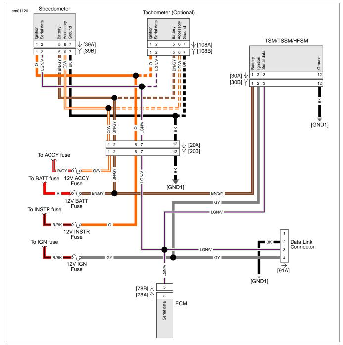
Figure 2-4. Serial Data Circuit
