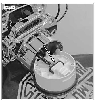
Figure 2-9. Speedometer Connector [39] (Typical)
