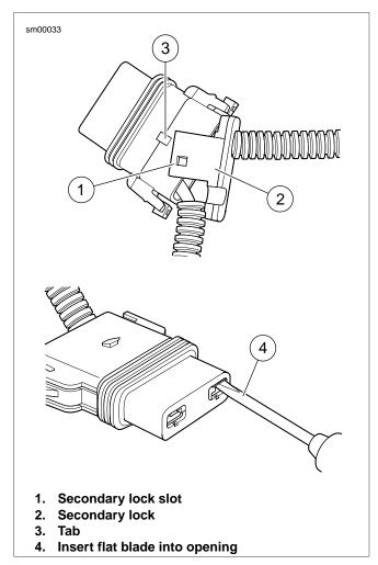
Figure A-31. Delphi Maxi-Fuse Housing: Remove Socket Terminals
