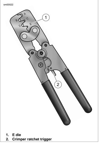
Figure A-20. Packard Terminal Crimper (HD-38125-7)
