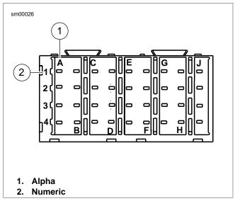
Figure A-24. Fuse Block: Coordinates (typical)
