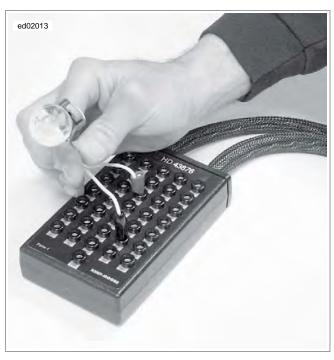
Figure 4-55. Ignition Coil Circuit Test
