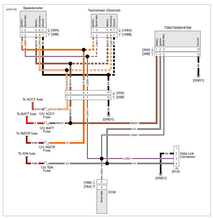
Figure 4-54. Serial Data Circuit
