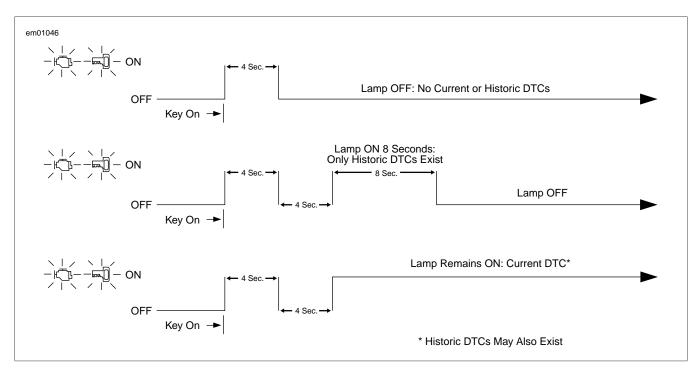
Figure 4-5. Check Engine Lamp Operation
