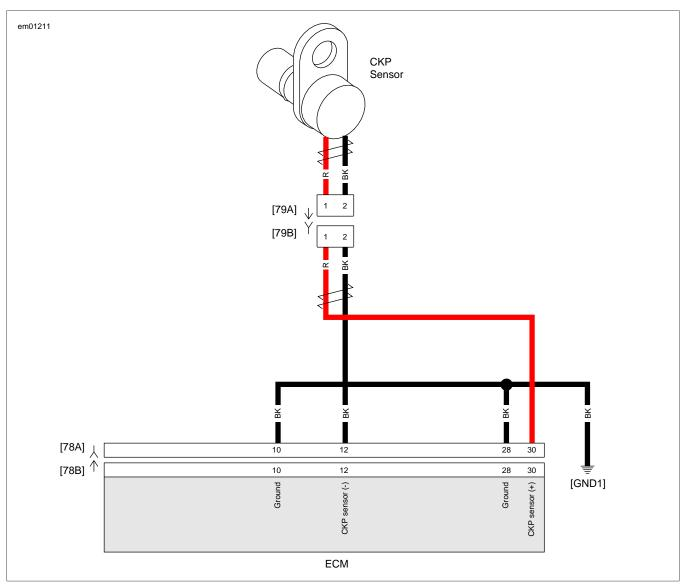
Figure 4-47. CKP Sensor Circuit
