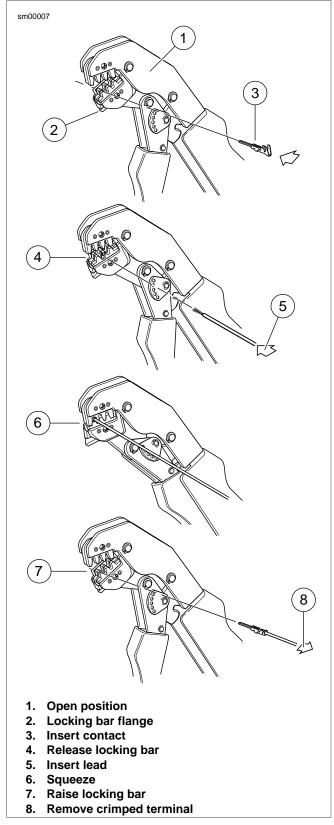
Figure A-8. AMP Multilock Connector: Terminal Crimping
