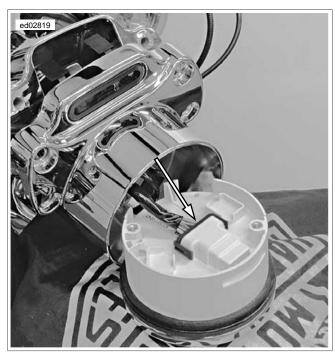
Figure 2-12. Speedometer Connector [39] (Typical)
