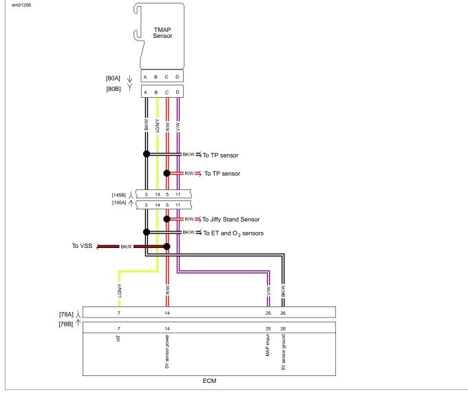
Figure 4-37. TMAP Sensor Circuit
