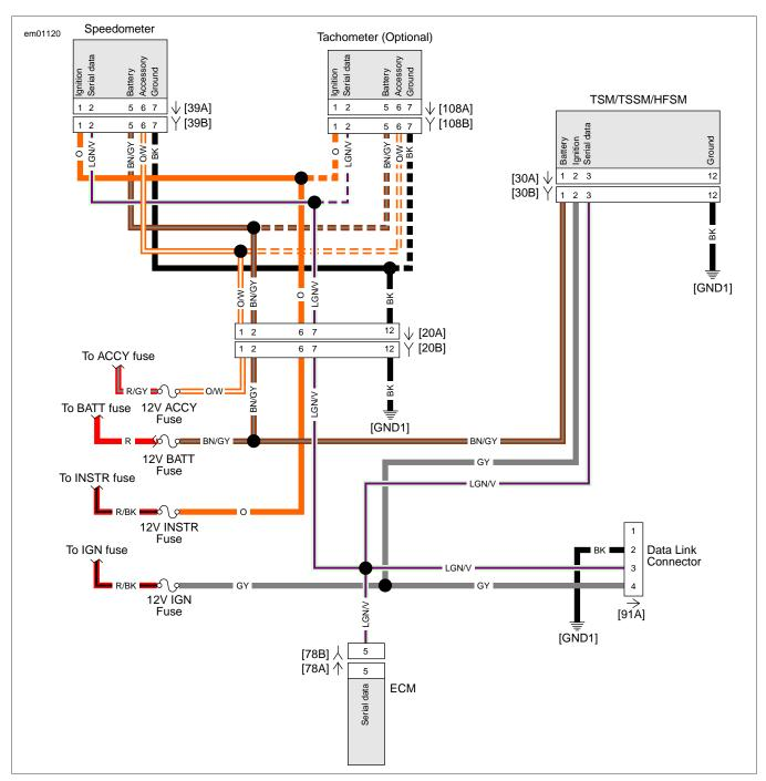
Figure 2-23. Serial Data Circuit
