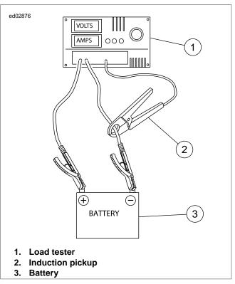
Figure 1-23. Load Test Battery
