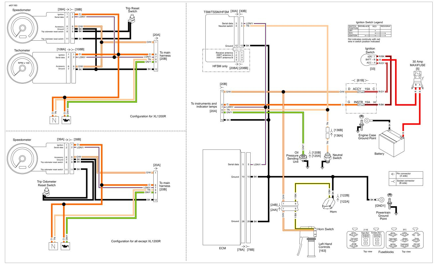
Figure B-9. 2008 SPORTSTER DOM. and INT. MODELS, HORN AND INSTRUMENTS
