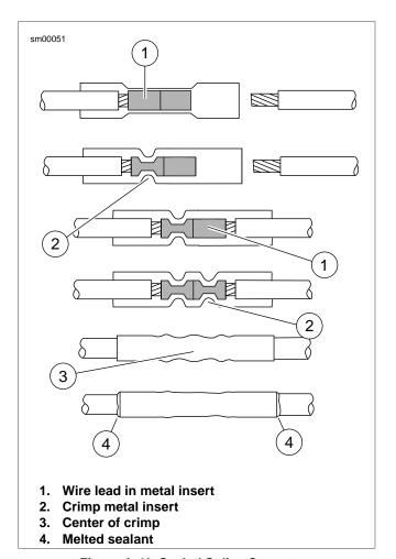
Figure A-49. Sealed Splice Connector
