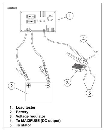
Figure 1-18. Current and Voltage Output Test
