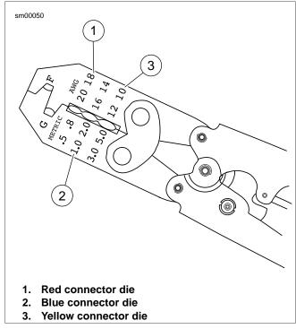
Figure A-48. Packard Crimping Tool (HD-38125-8)
