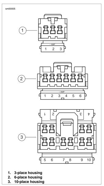
Figure A-5. AMP Multilock Connector: Cavity Numbers on Secondary Locks (Socket Housings Shown)
