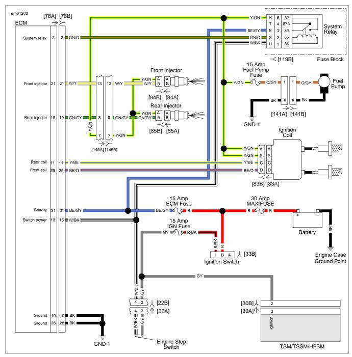
Figure 4-25. System Relay Circuit
