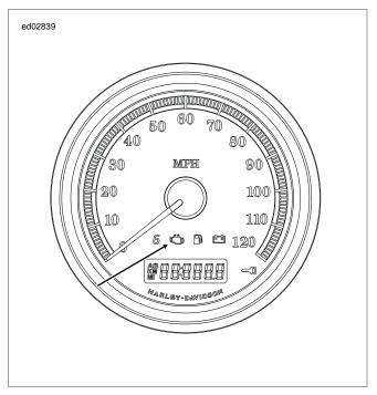
Figure 4-3. Check Engine Lamp
