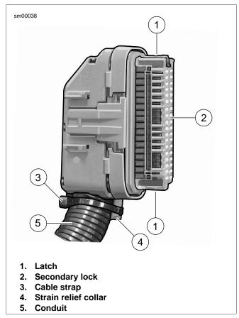
Figure A-41. Packard 100W Connector
