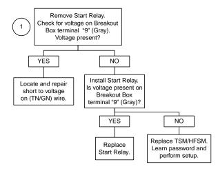
Clear DTCs using speedometer self diagnostics. See 3.11 SPEEDOMETER SELF DIAGNOSTICS. Confirm proper operation with no check engine lamp.
