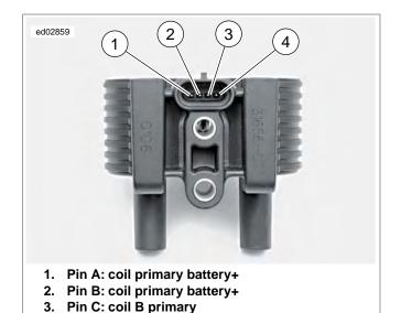
Figure 4-56. Ignition Coil Connector Terminals
