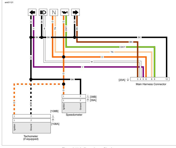
Figure 2-11. Indicator Lamp Circuitry
