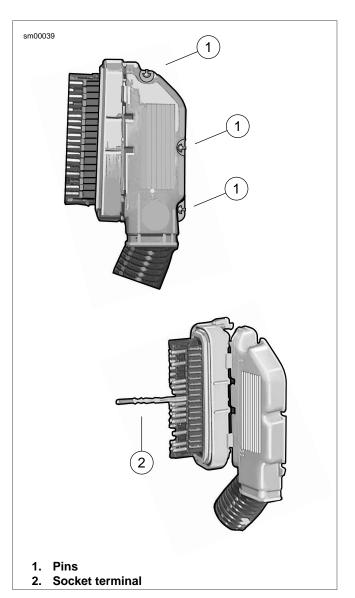
Figure A-42. Packard 100W Connector: Separate Halves of Socket Housing
