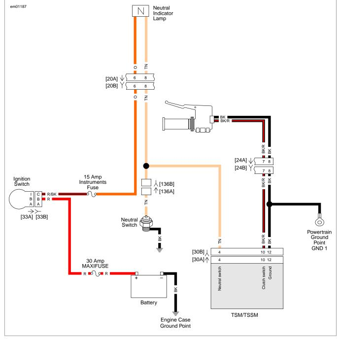
Figure E-25. Clutch and Neutral Interlock Circuits
