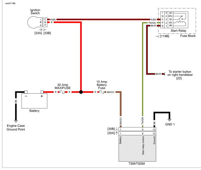
Figure E-24. Starter TSM/TSSM Circuit
