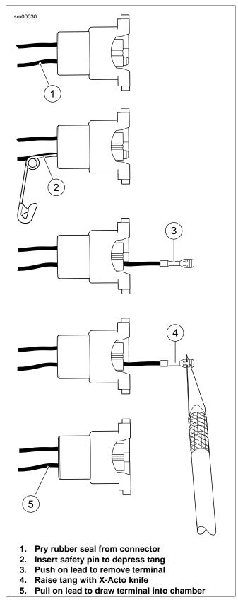
Figure A-28. 280 Metri-Pack Connector: Remove/Install Socket Terminal
