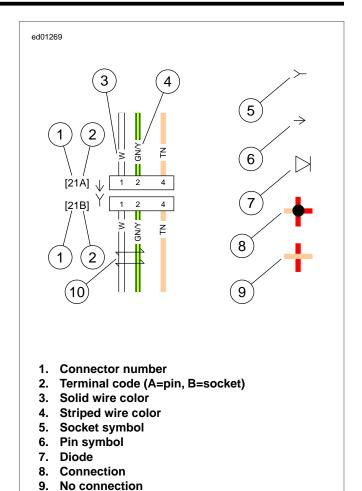
Figure B-1. Connector/Wiring Diagram Symbols (typical)
