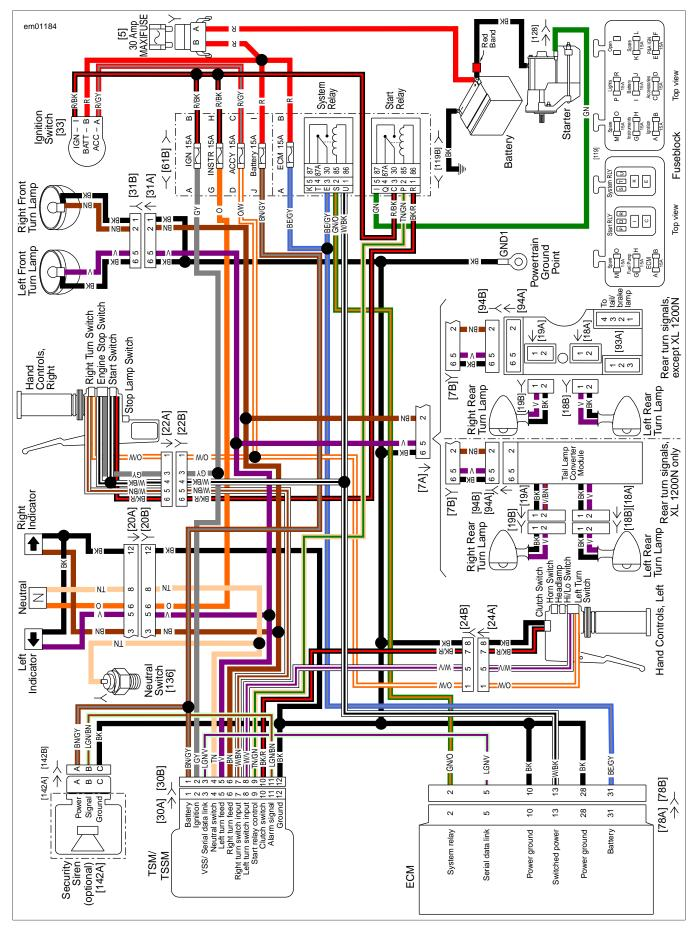
Figure E-19. Turn Signal Circuit: Typical
