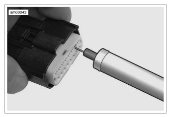
Figure A-38. Molex Connector: Terminal Remover (HD-48114)
