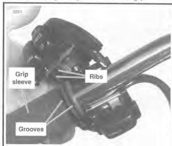
Figure 7-75. Install Left Handlebar Switch Housings
