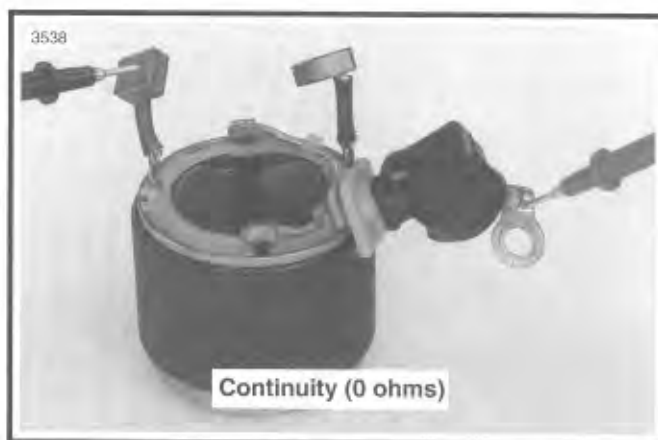
Figure 5-18. Open Field Test
