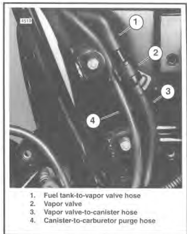
Figure 4-21. Vapor Valve and Hose Routing - California
