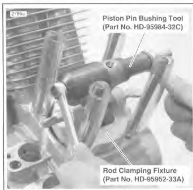
Figure 3-36. Installing New Piston Pin Bushing
