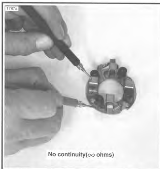
Figure 5-19. Brush Holder Insulation Test
