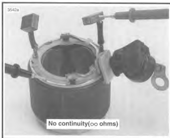
Figure 5-17. Grounded Field Test
