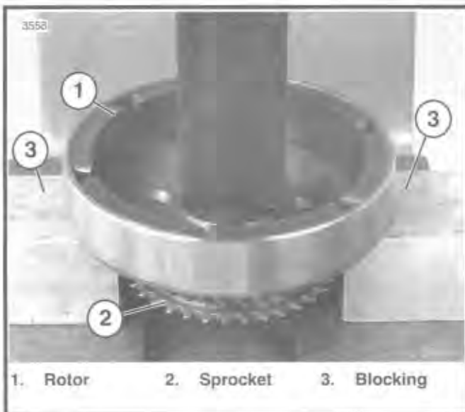
Figure 7-47. Removing Rotor From Sprocket
