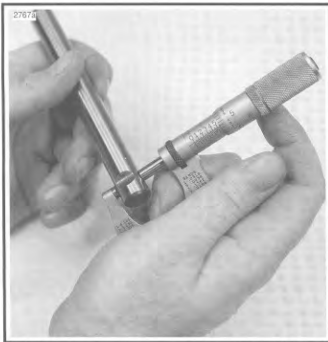
Figure 3-11. Measuring Rocker Arm Shaft Diameter (Rocker Cover Position)
