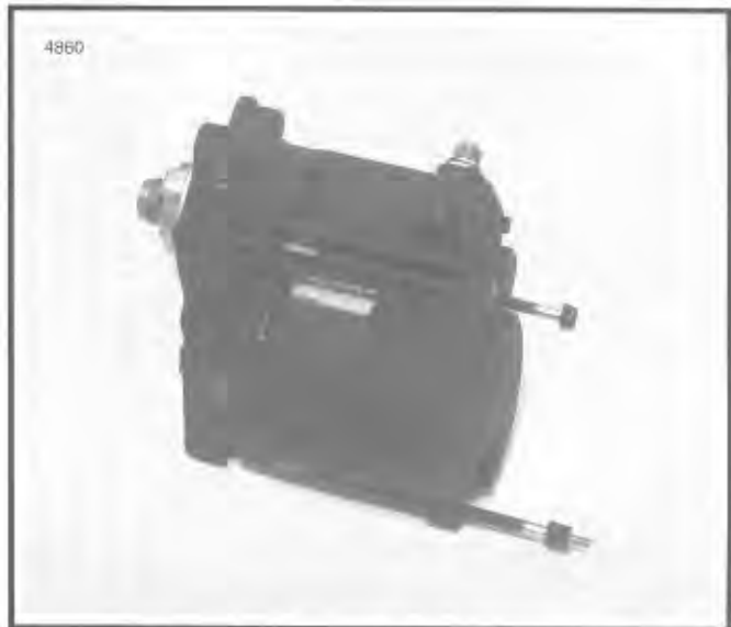
Figure 5-9. Removing the Thru-Bolts
