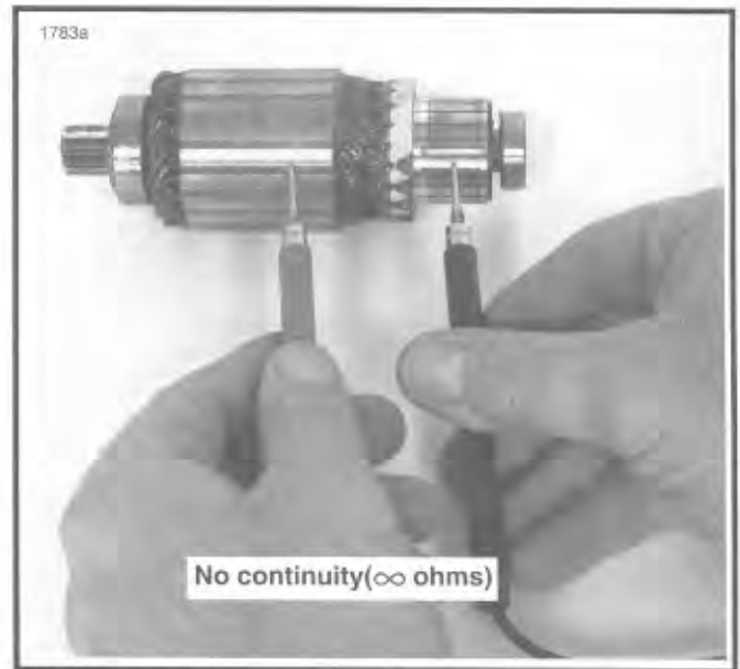
Figure 5-15. Grounded Armature Test
