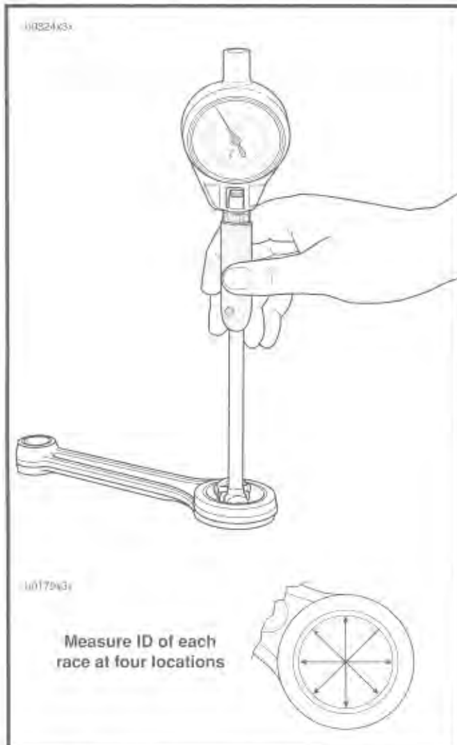
Figure 3-82. Measuring Connecting Rod Race Inside Diameter
