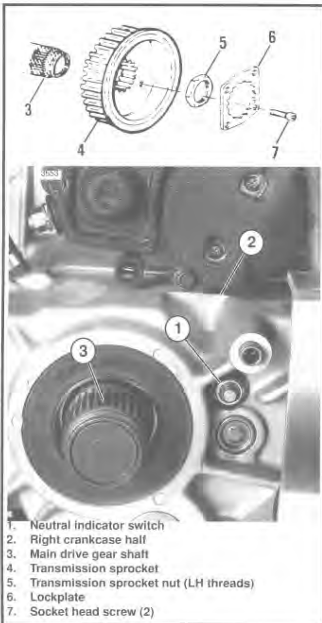
Figure 7-85. Neutral Indicator Switch
