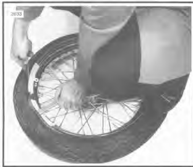
Figure 2-33. Starting Tire Off Rim
