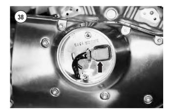
3. Spray the sensor (**Figure 38**) with a refrigerant (available at electronic supply stores). If the engine dies, replace the sensor as described in Chapter Twelve.
