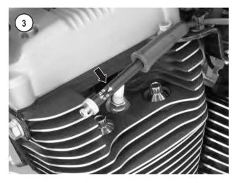
3. Insert the spark plug (**Figure 2**), or spark tester (**Figure 3**), into its plug cap and ground the spark plug base against the cylinder head. Position the spark plug so the electrode is visible.
