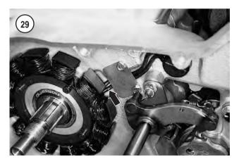
3. Do not operate the start switch if the ignition module is not grounded. The black ignition module wire is the ground wire. Inspect the wire end for corrosion and damage. Be sure the ignition module is mounted securely.
