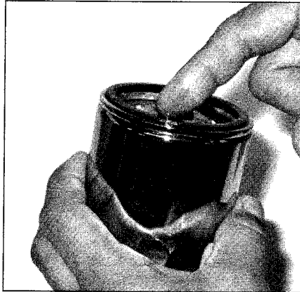
9.9 Smear a film of clean oil onto the gasket surface
