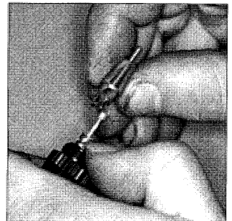
6.67b . . . then slip the cable end out of the plunger to separate the plunger from the cable (Keihin CV carburetor)
