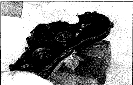
5.8 Tapping a casing face down on wood blocks can often dislodge a bearing
