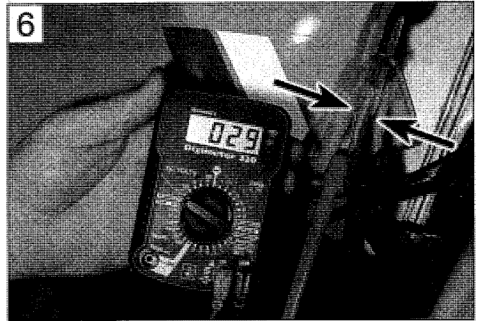
6 Continuity check of front brake light switch using a meter - note cotter pins used to access connector terminals
