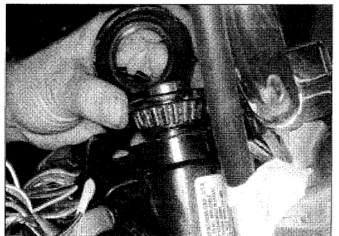
5.9b Lift off the bearing cover and upper bearing
