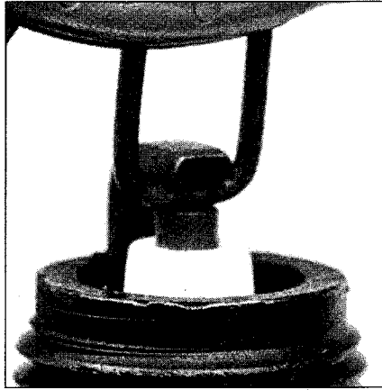
26.5a Spark plug manufacturers recommend using a wire type gauge when checking the gap - if the wire doesn't slide between the electrodes with a slight drag, adjustment is required
