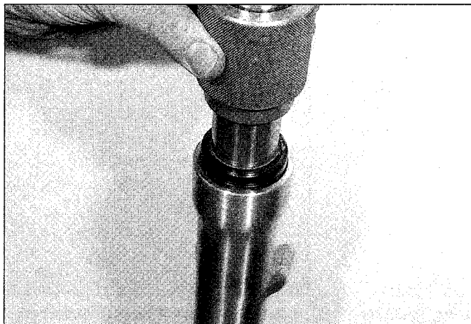
4.28n Use any of the tools previously shown to drive the dust seal (1984 and later) into place
