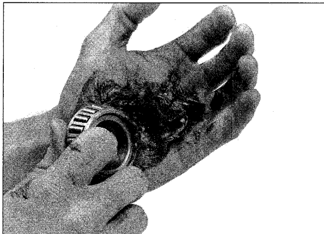
5.15 Work the grease completely into the rollers
