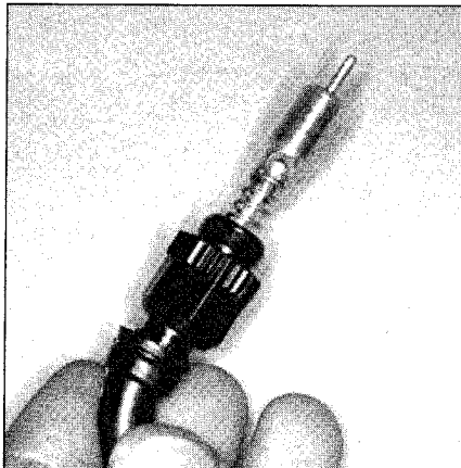
6.67a Unscrew the starter valve from the carburetor and compress the spring . . .
