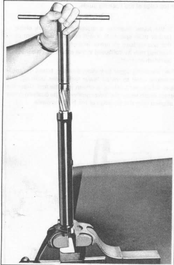
Figure 2-48. Reaming Fork Slider Bushing
