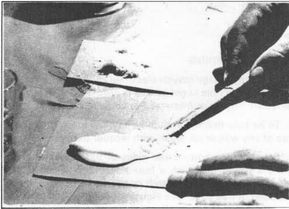
Figure 2-67. Mixing Gel Coat Glass Fibers
