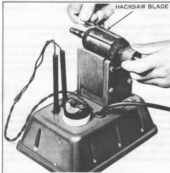
Figure 5-15. Testing Armature for Short
