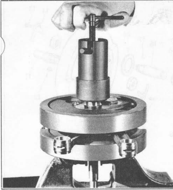
Figure 3-43. Removing Bearing from Sprocket Shaft
