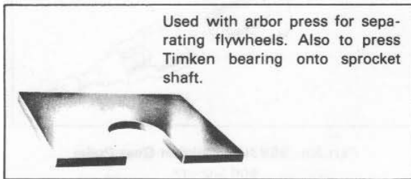
Part No. 96137-52A Flywheel Support Plate
