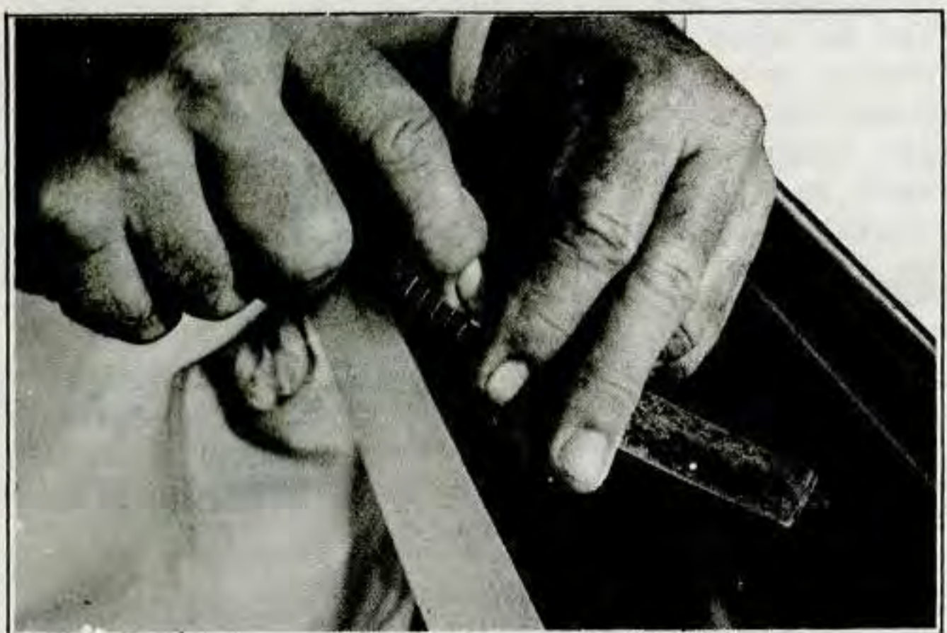
Figure 2J-4. Trimming Patch
