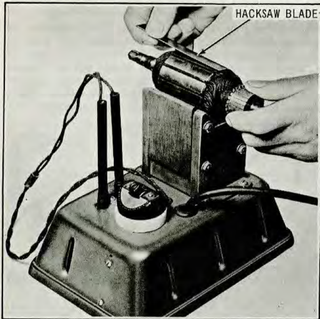
Figure 5E-4. Testing Armature for Short
