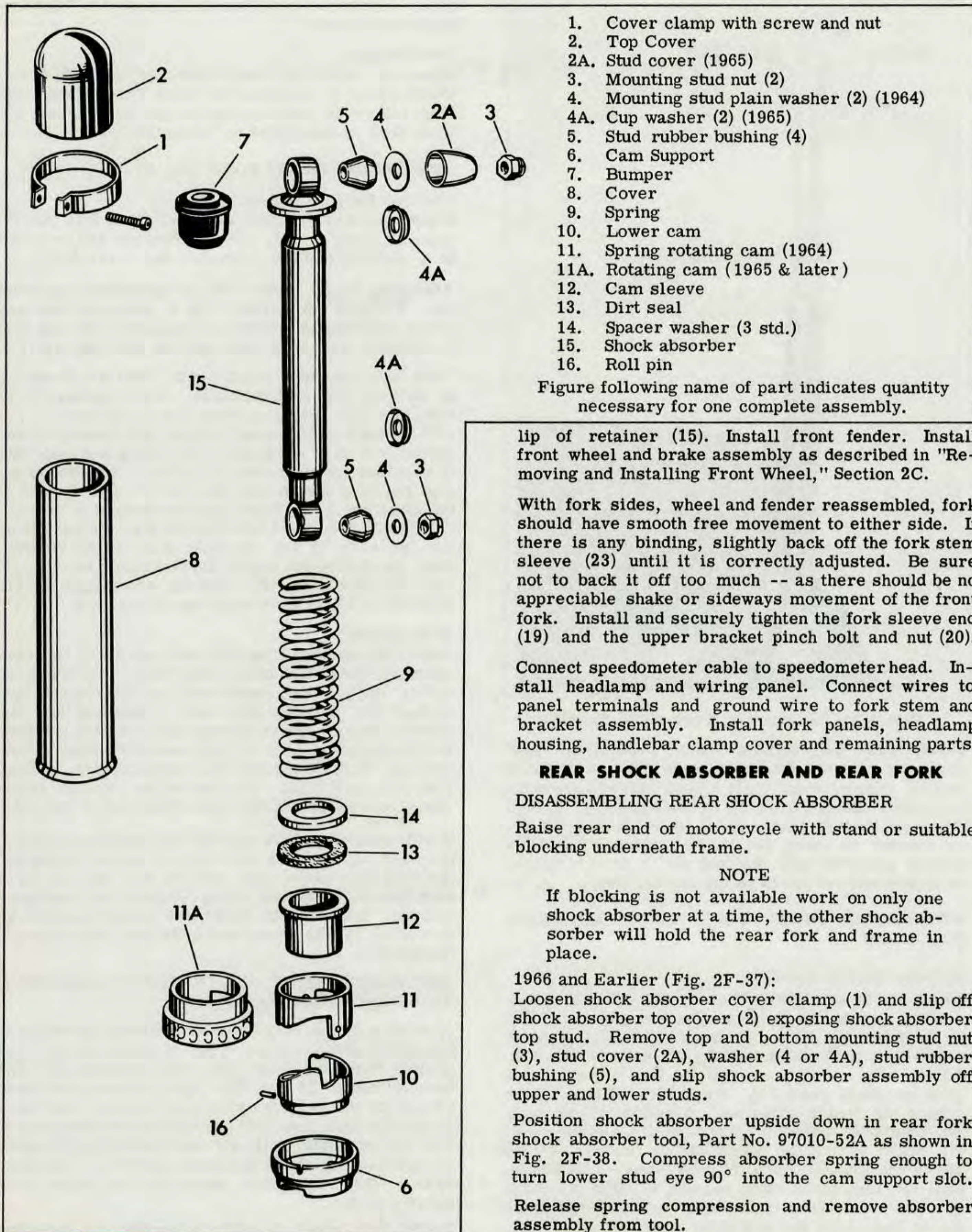
Figure 2F-37. 1966 & Earlier Rear Shock Absorber - Exploded View
