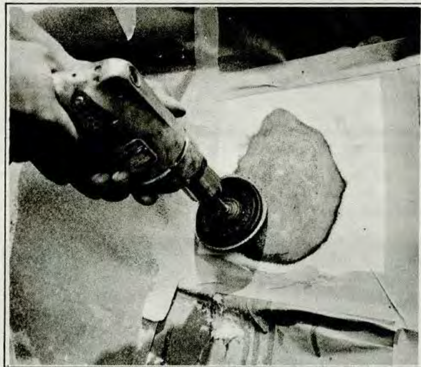
Figure 2J-13. Blending Patch with Sander
