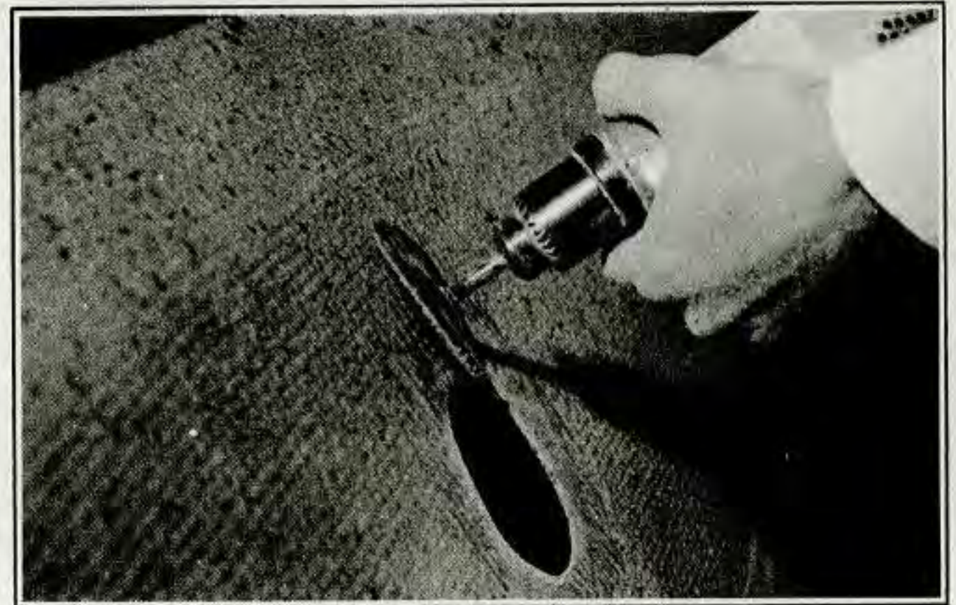
Figure 2J-8. Rough Sanding Inside Surface
