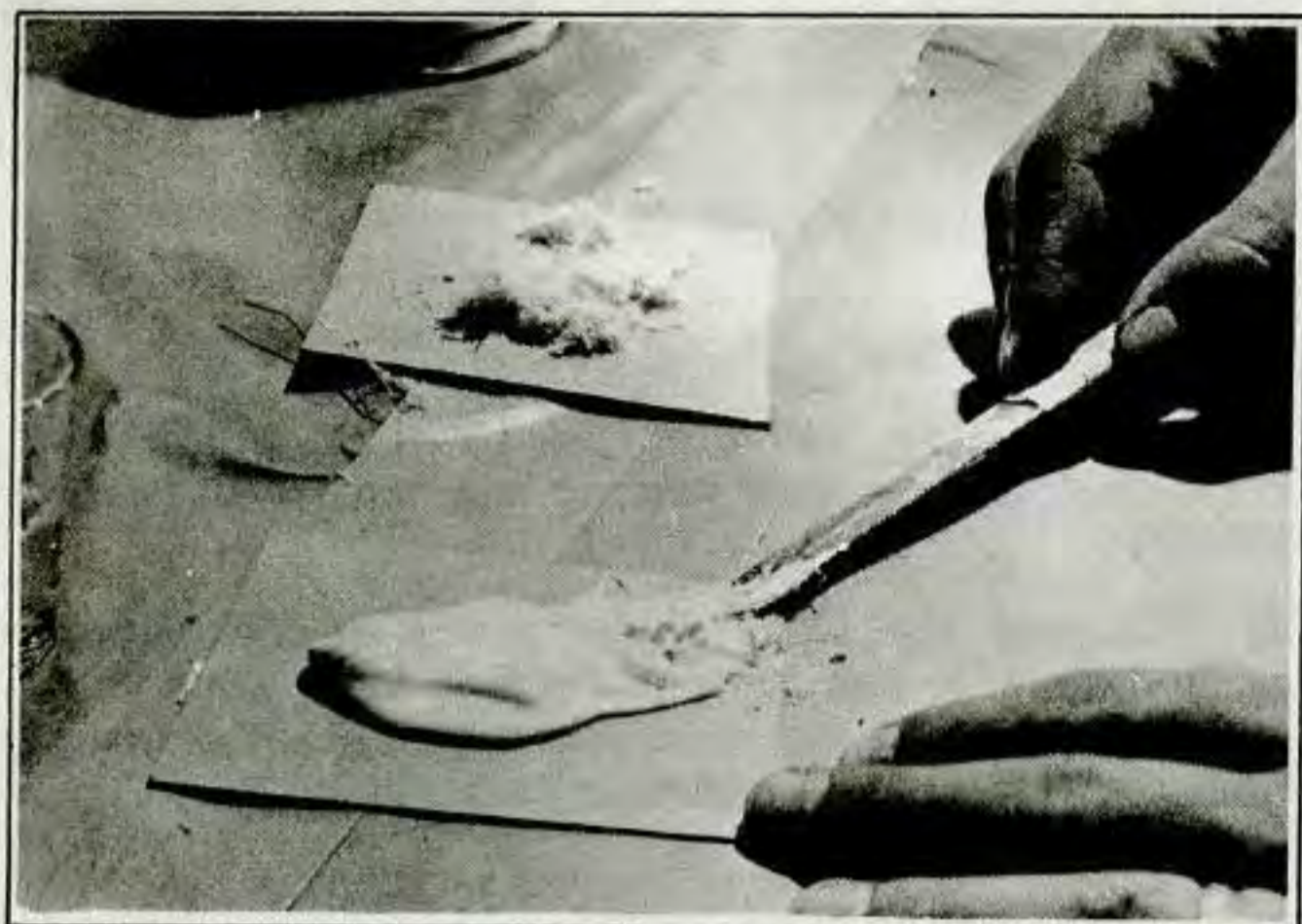
Figure 2J-2. Mixing Gel Coat and Glass Fibers
